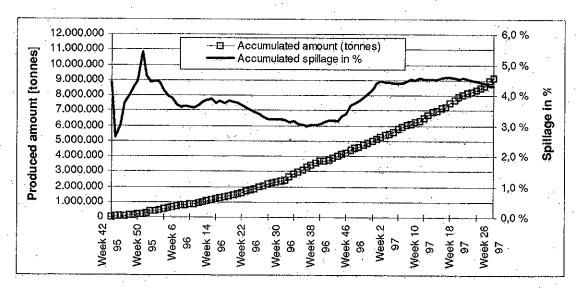
Fig. 2. Development over time of the total production quantity in tonnes and the accumulated spillage in per cent for the dredging work as a whole. Source: Oresundskonsortiet.
