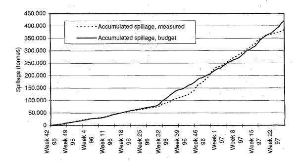
Fig. 3. Development over time of the measured spillage from the dredging and extraction work up to the end of June 1997 in relation to the budgeted spillage for the period.
