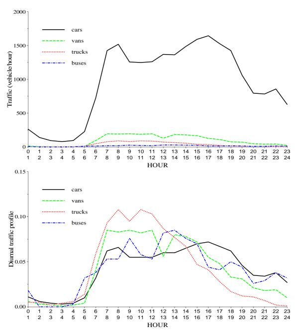
Figure 17 Average working days diurnal variation of traffic at Jagtvej; a) traffic flow, b) diurnal profile.
