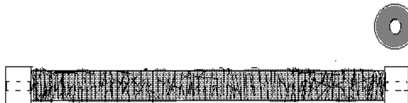
Yarn-wound on aluminum housing 20mmØx250mm
