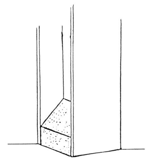
Cement filling provides easy cleaning and prevents pests
