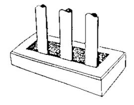
C<u>orrect:</u> enables cleaning dust e.g. is not accumulated W<u>rong:</u> difficult to clean dust is accumulated harborauge for pests
