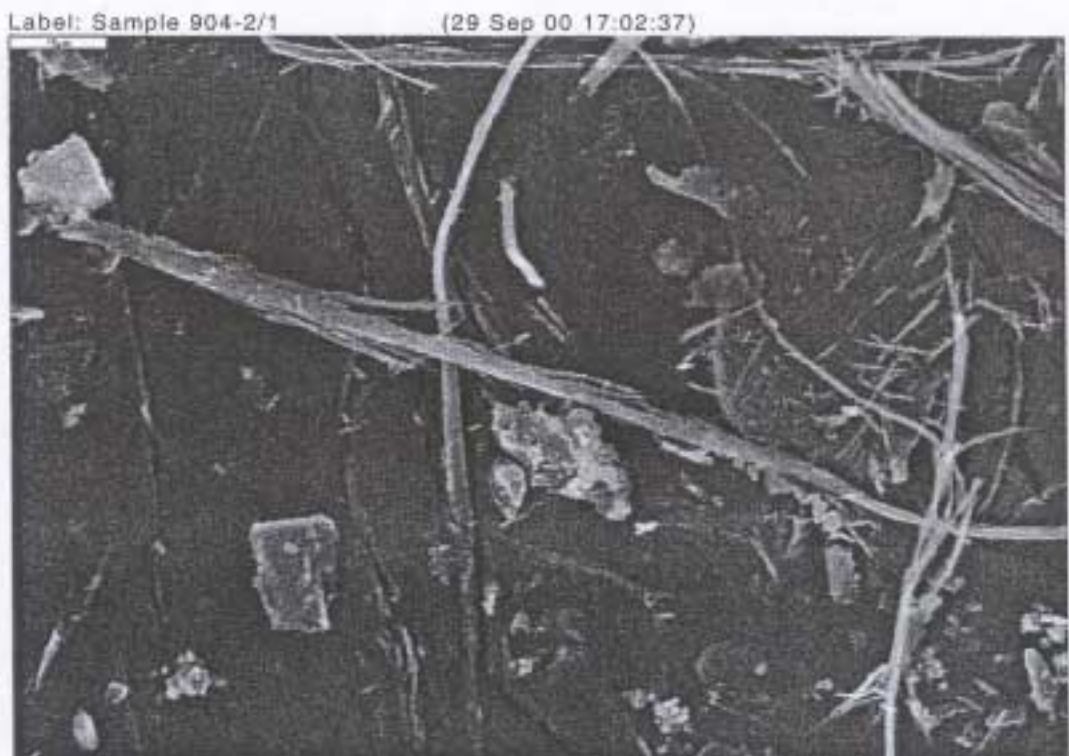
Fig. 6B. Sample no. 904-2. Fibres of sepiolite. SEM. Magnification 5000 times.
