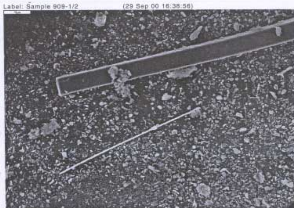
Fig. 7B Sample no. 909-1. Fibres of nemalite. SEM. Magnification 5000 times.
