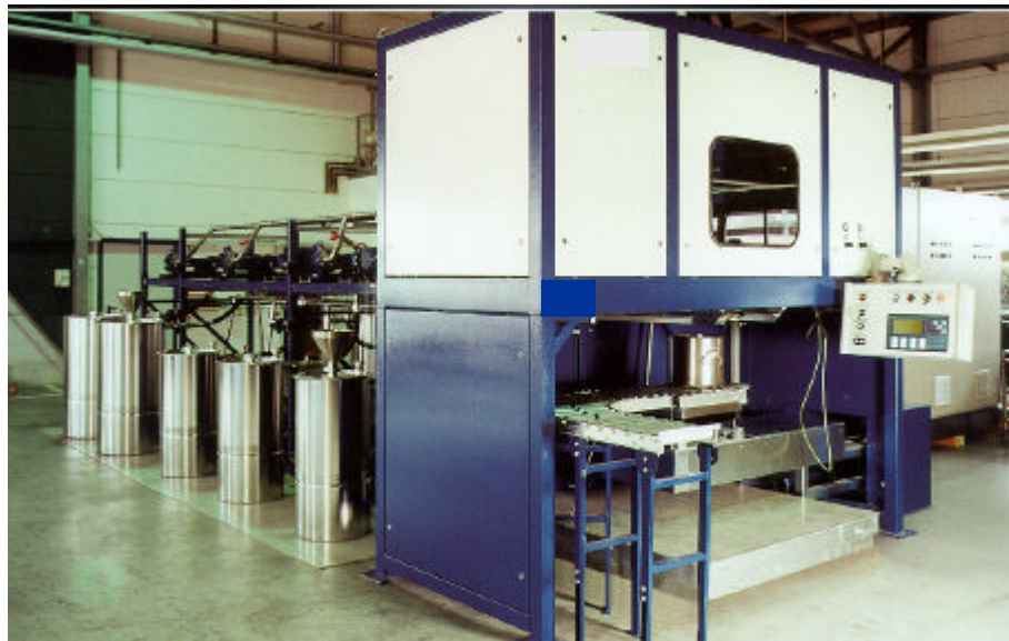
Photo 17: Automatic filling station.
