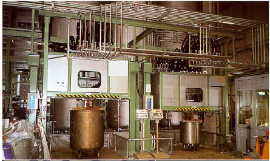
Photo 3: Dosing station for mobile bins (semi-closed).
