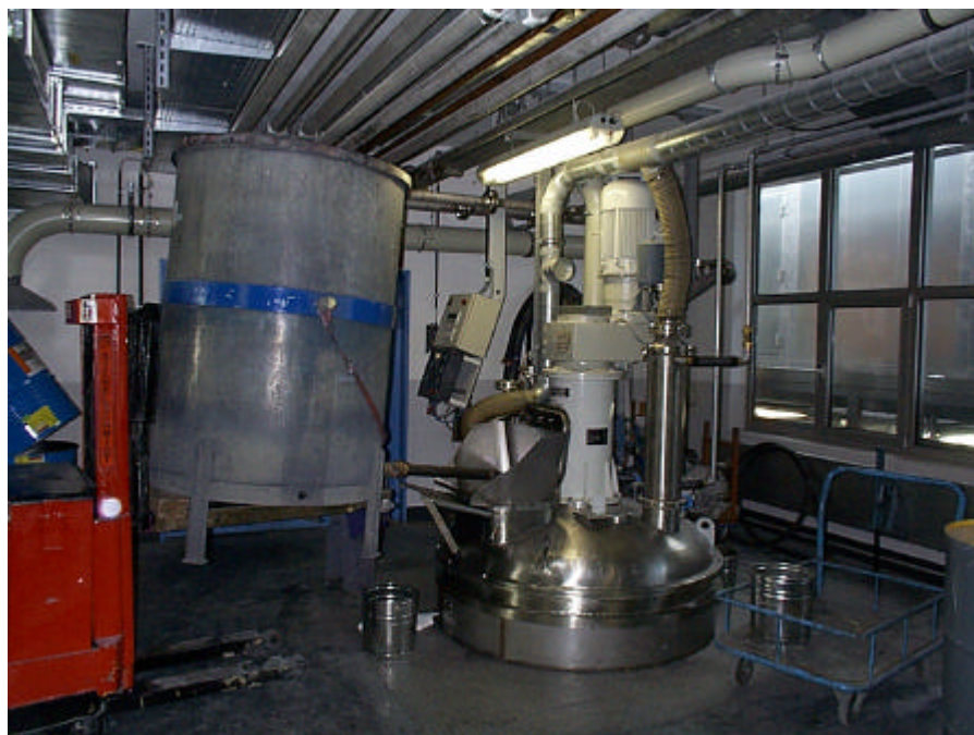
Photo 1: Dosing of liquid raw material into a Dissolver, condensation system and flexible hose system on the dissolver lid.
