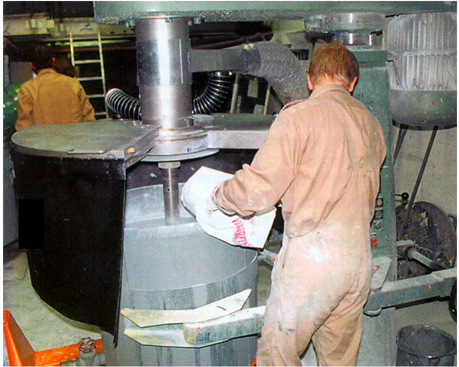
Photo 11: Dissolver encapsulation with possibilities for manual addition of powder.
