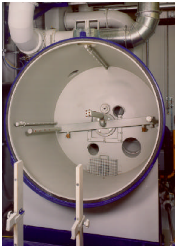
Photo 4: Washing machine type SKM for inside and outside cleaning by spray (Renzmann).
