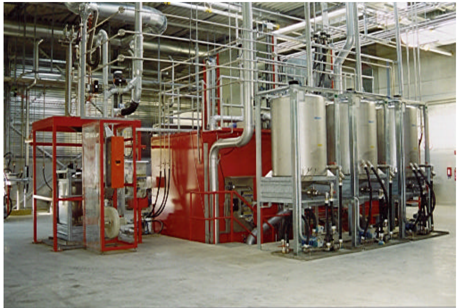
Photo 15: Special washing tanks for transparent and isocyanate coatings (Riobeer).
