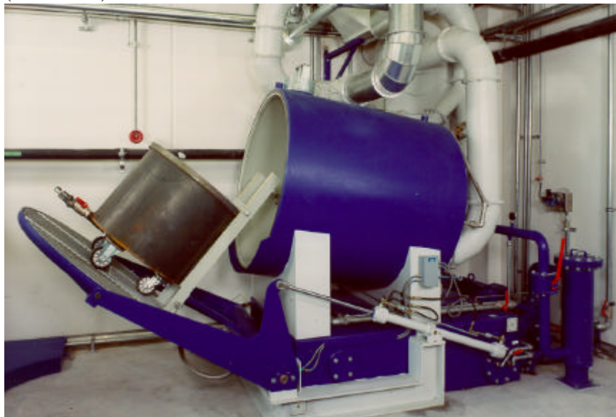
Photo 3: Washing machine type SKM for inside and outside cleaning by spray (Renzmann).
