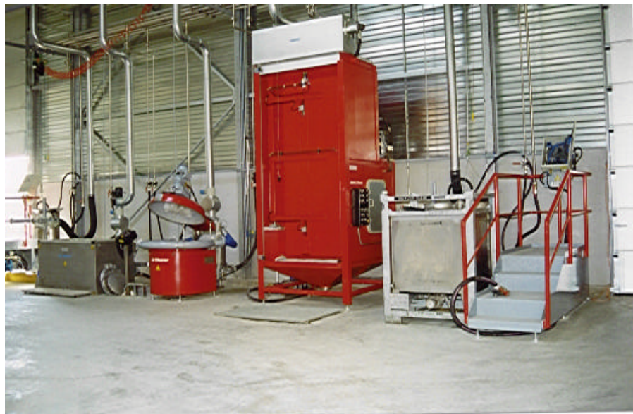
Photo 10: Additional equipment (from left): Precleaning station, manual cleaning station, lid cleaner, agitator cleaner, precleaning station (Riober).
