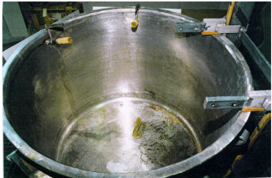
Figure 2 Mixing vessel after cleaning in SKM plant (Stripper 303 G/E, 80°C, 12 minutes).
