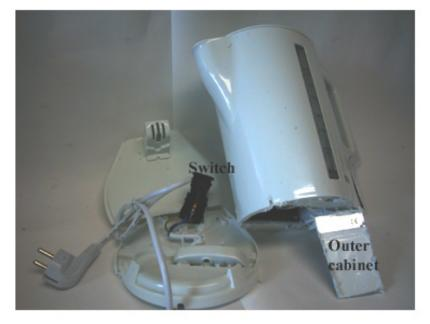
Project: Bromine in Electronic Parts Encl. A-11 Tefal Boiling Pot
