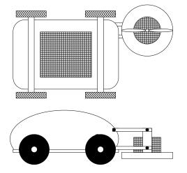
Figure 8.4. Outline of large beetle type weeder with front mounted rotor cutter. A wide design is proposed to place the wheel traffic in the cut lanes only.
