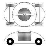
Figure 8.3. Outline of small "beetle type" ACW mounted with central placed rotor cutter.
