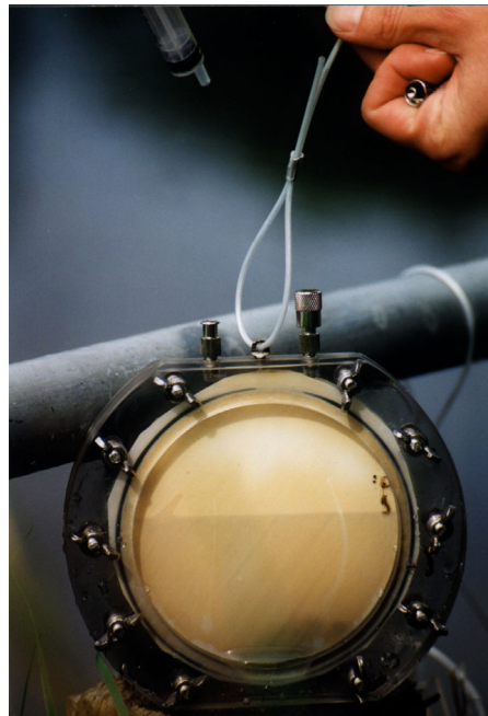
Figure 2.2. A membrane-filter chamber used in the in situ pond experiment.
