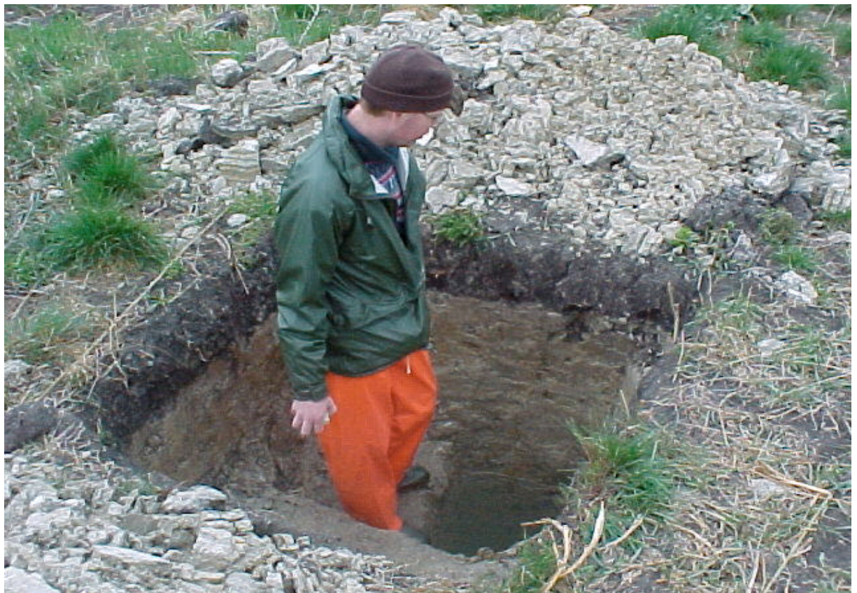
Test pit for soil characterisation at the experimental site at Roma. (Photo: Stig Larsson)
