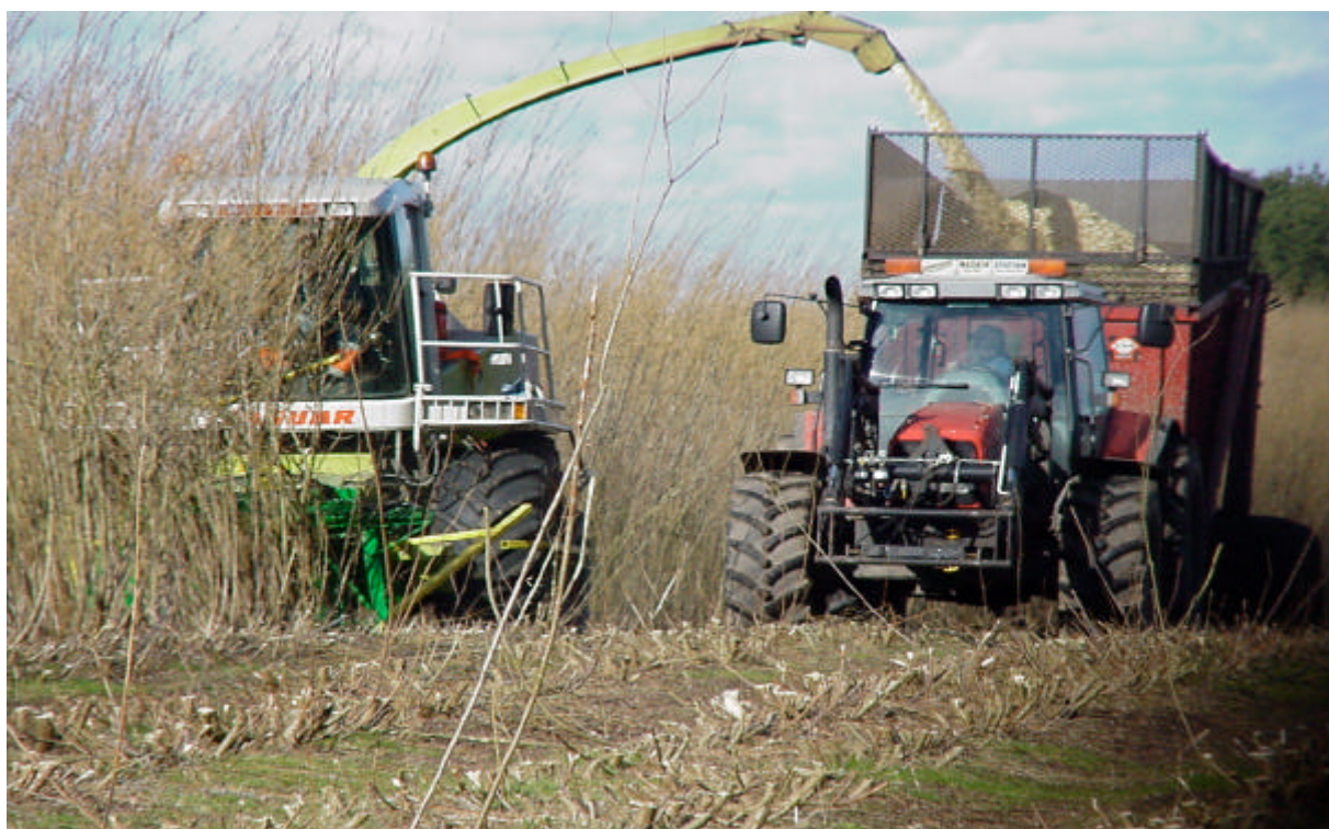
Combined harvesting and chipping of a willow plantation in Sweden. (Photo: Stig Larsson)
