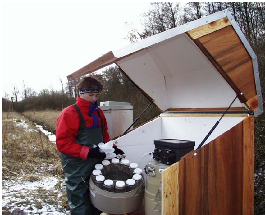
Photo 3.1. ISCO-sampler in sampling house at stream monitoring station in the Odderbæk catchment.
