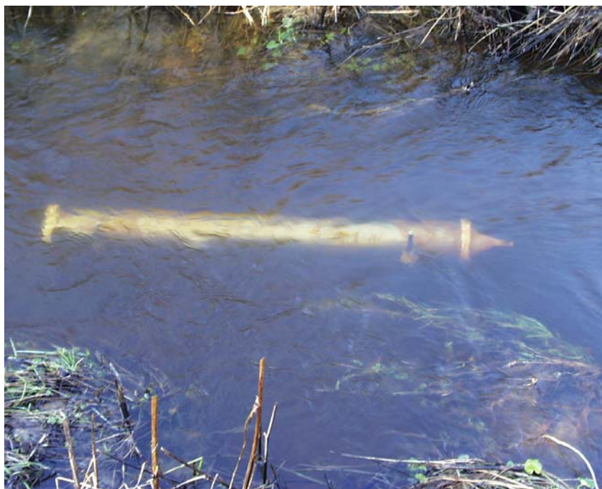
Photo 3.3 prototype of the suspended sediment sampler installed in Oddebæk in December 1999.
