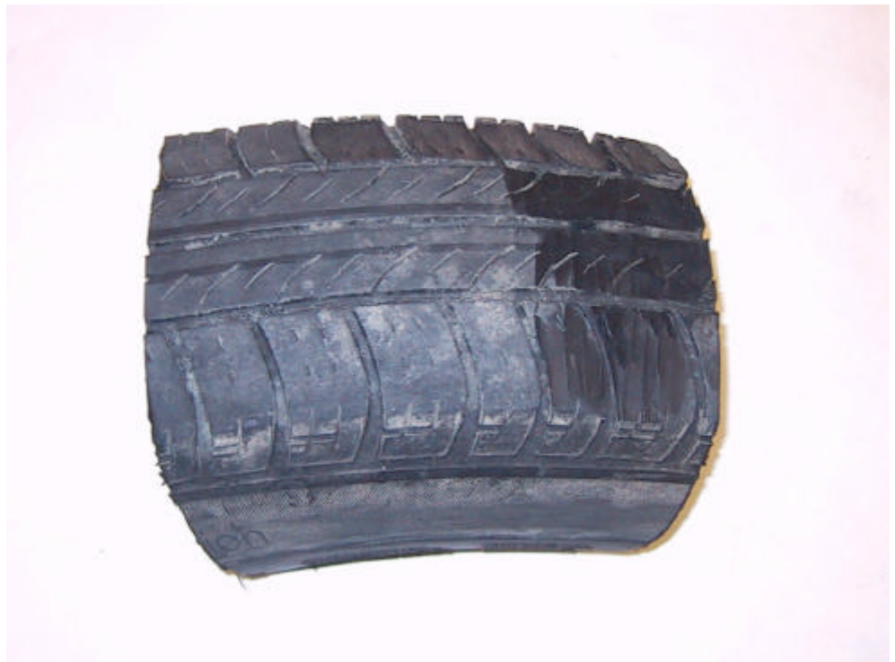
Passenger car tyre, sampling from tread
