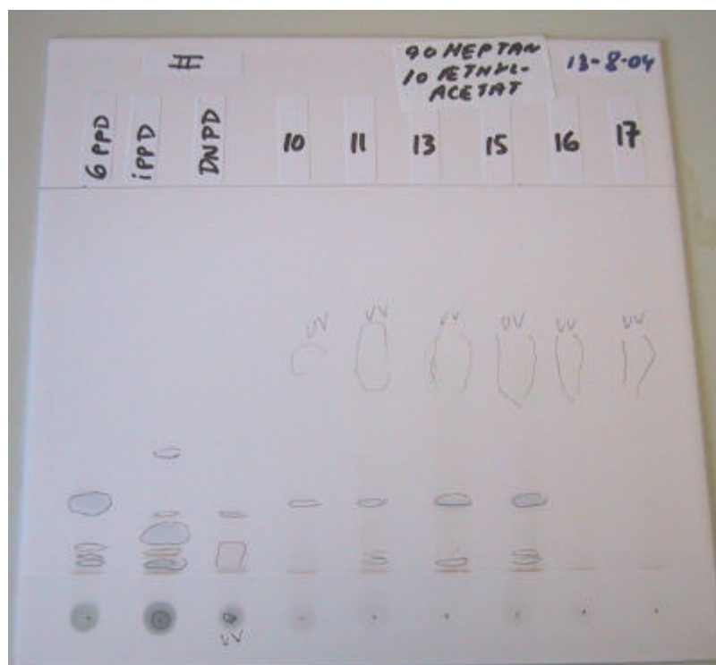
TLC screening for aromatic amines before iodine treatment
