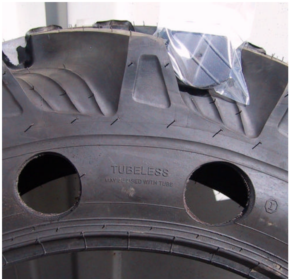
Tractor tyre, sampling from side wall
