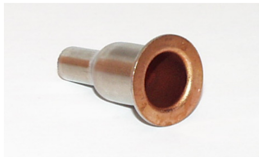
Figure 2.5 The three work pieces are made in a step press at Danfoss A/S with up to seven draws and a final calibration (extrusion to final thickness of material). The materials are stainless steel (W.nr. 1.4301), acid resistant steel (W.nr. 1.4404), and a copper coated acid resistant steel ((W.nr. 1.4404 / Cu).
