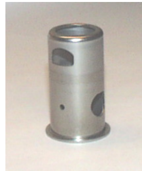
Figure 2.4 Deep drawing in several steps with slight extrusion in final step. Performed in a multistage deep drawing including slight extrusion in the last step. Produced in a step press. 0,8 mm stainless steel (W.nr. 1.4306)
