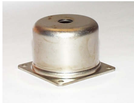
Figure 2.4 Deep drawing in several steps with slight extrusion in final step. Performed in a multistage deep drawing including slight extrusion in the last step. Produced in a step press. 0,8 mm stainless steel (W.nr. 1.4306)
