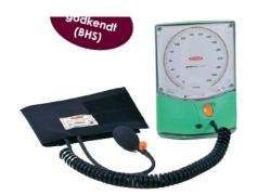
EXAMPLE: Greenlight 300 electronic sphygmomanometer with manual reading, marketed as reference manometer. Using the auscultatory techniques and electronic manometer. Self calibrating when switched on. Meet the criteria of the International Protocol for blood pressure measuring devices in adult (BHS 2006) (Manufacturer: AC Cossor & Son (Surgical) Ltd., UK).
