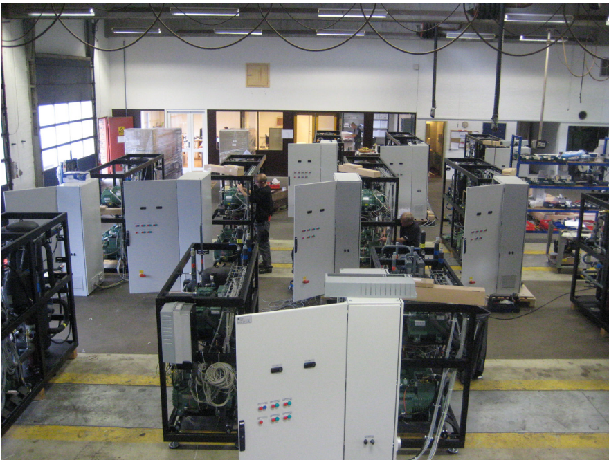
Photo 5: Photo from the production of “remote refrigeration packs” for CO 2 at the Advansor Company in Aarhus.
