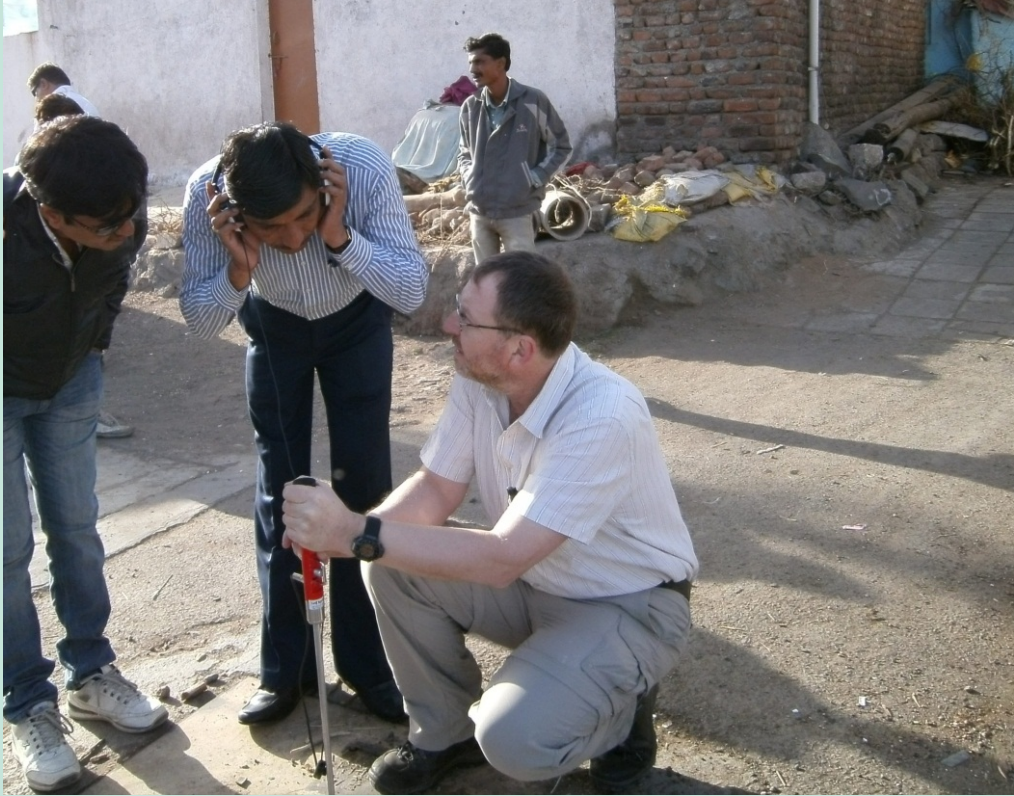
FIGURE 4 LISTENING TO WATER LEAKING IN THE WATER SUPPLY SYSTEM IN RAJKOT CITY, GUJARAT STATE, INDIA
