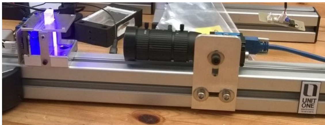
Figure 5. Setup of a simple test system with an industrial video camera (1600 x 1200 pixels, 1/1.8" CCD sensor, 4,4µm pixel size) and a zoom lens. On the left side is the light source, and holder for a cuvette with the sample volume.
