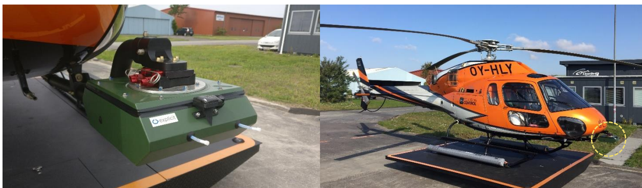
Image B and C The snifferbox mounted on an AS355NP equipped with a carrying arm.
