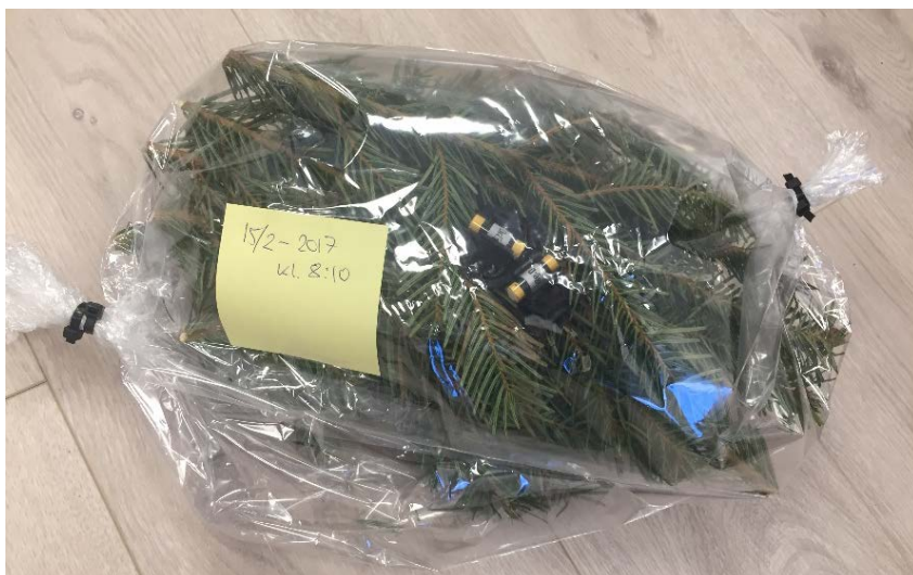
FIGURE 3.7. Nalophane bag containing Nordmann fir branches and two ORSA-samplers for the Fir Study.
