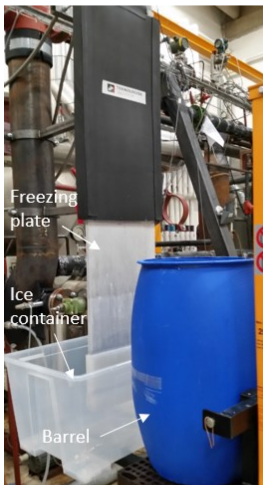
Figure 11. Test setup for freeze concentration
