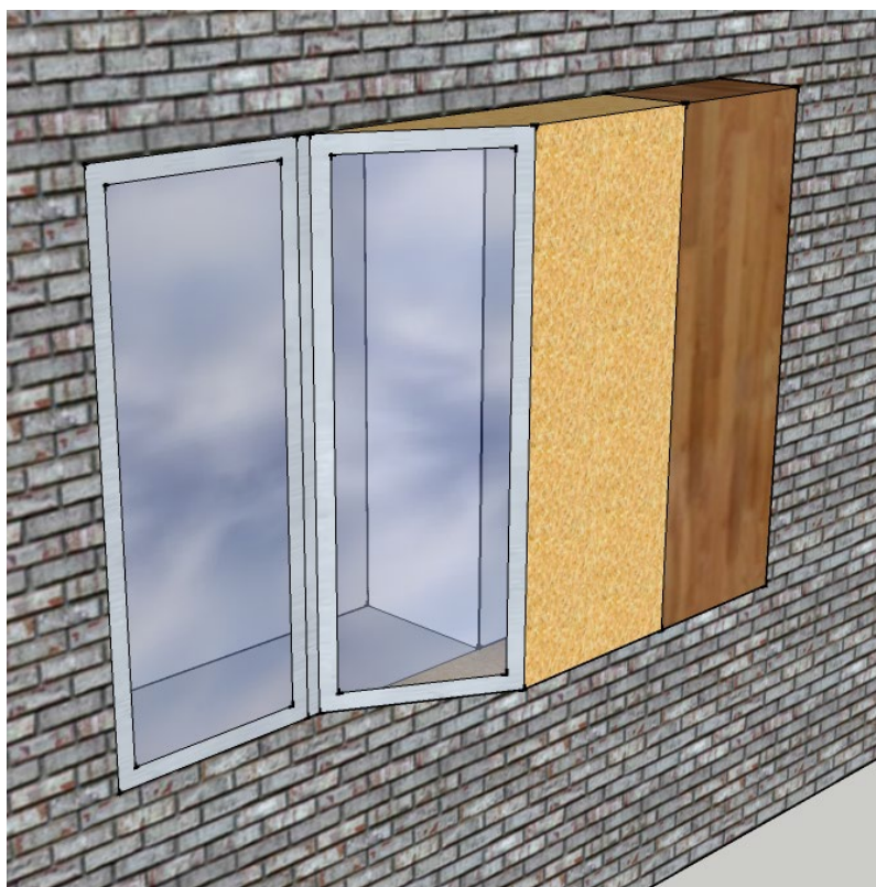
Illustration 9J. Sketch of mockup solution C. The construction is here shown with two different brown patterns, where the light part marks the default construction, and the dark part marks the extension which was also investigated. Both parts (including the parallel wall) can be covered by absorber.
