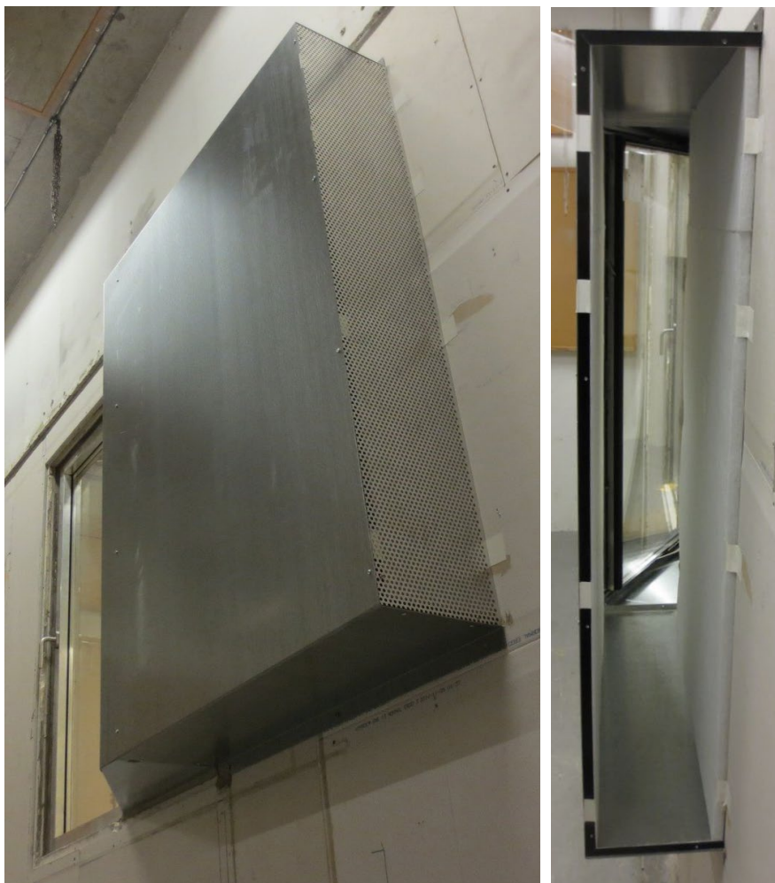
Illustration 9M Photo from the outside of the prototype. Left photo shows the construction from below, where the bird grate can be seen. Right photo shows the construction from the opening in the prototype, where 20 mm absorber is added to the top, bottom and sides. See additionally Illustration 9A.
