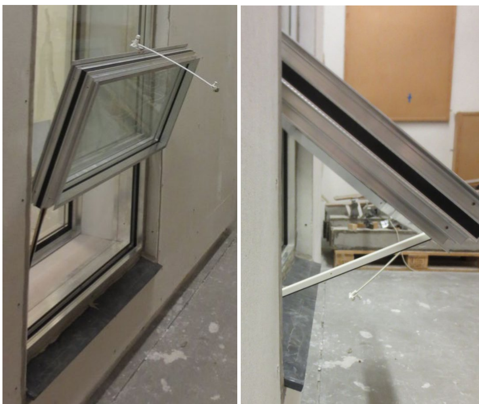
Illustration 10H. Photo from the laboratory measurements taken from the external side. Left photo shows the vent opened as much as possible, while the right photo shows the vent in a “diagonal position”. In both situations the opening area is approximately 0.35 m 2 .
