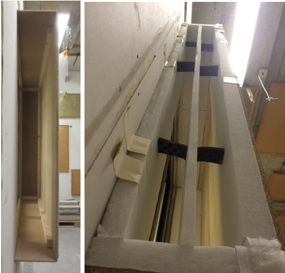
Illustration 9G. Two photos of mockup solution B, both taken from the open end of the construction. Left photo shows the construction without added absorber. Right photo shows the highest amount of added absorber investigated during the measurements, which is 40 mm in top, bottom and sides plus extra 20 mm in the middle.
