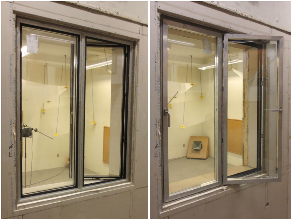
Illustration 9B. Photos of the applied "ordinary windows". Left photo shows a two-winged side hung window opening inward, with the hinges in the frame. Right photo shows a two-winged side hung window opening outward, with the hinges in the center.
