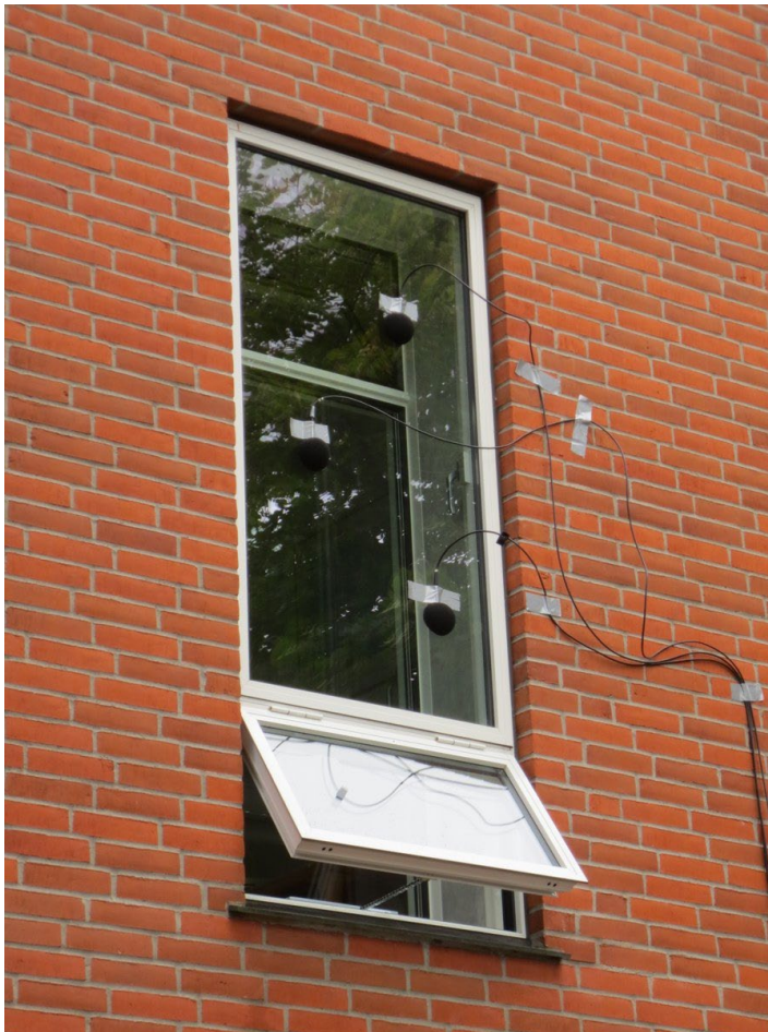
Illustration 10C. Photo from the field measurements, where the vents are opened as much as possible. The three microphones are mounted on the glass.
