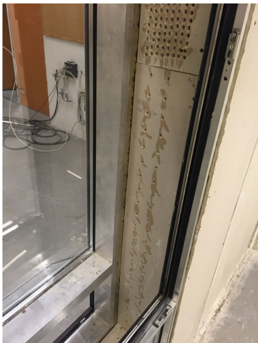
Illustration 7F. Photo of the window with respectively 34.91 % (upper) and 3.14 % (lower) perforated frame. The photo shows the lower part of the window.
