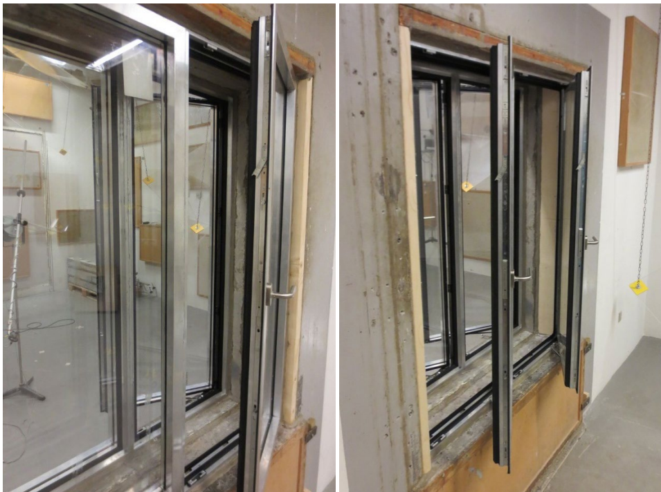
Illustration 8D. Photos of the window when open. Left photo shows the window opened as a two-winged side hung window, while the right photo shows the window with all the sashes opened.
