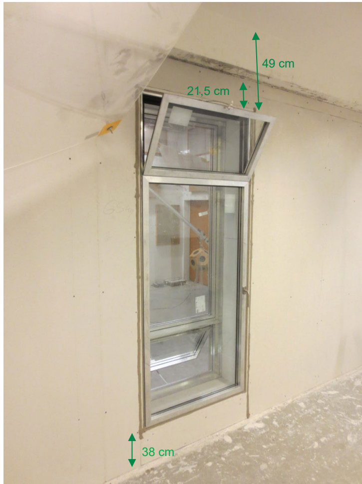
Illustration 10E. Photo from the laboratory measurements taken from the inside. The vents are “fully open”.
