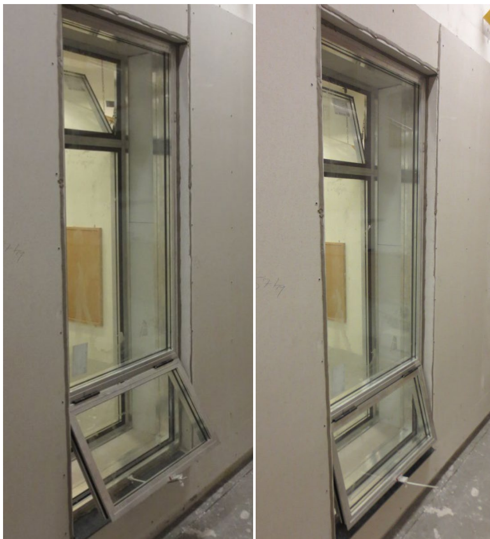
Illustration 10F. Photo from the laboratory measurements taken from the outside. Left photo shows the vents “fully open”, while the right photo shows the vents “4 cm” open.
