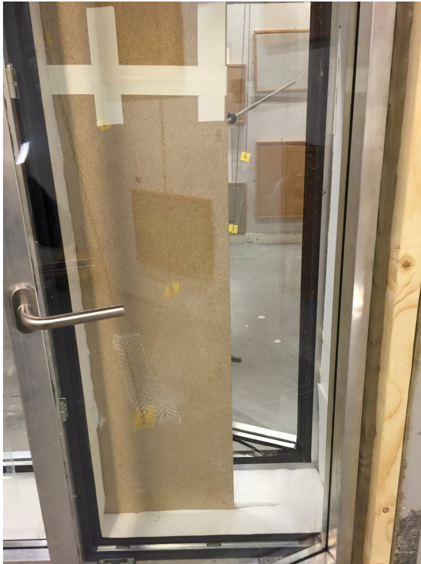
Illustration 8I. Photo of two-winged solution during measurement. Absorbers can be seen on both the plate in the middle and in the frame (both in the side and in the bottom), but not on the transverse plate.
