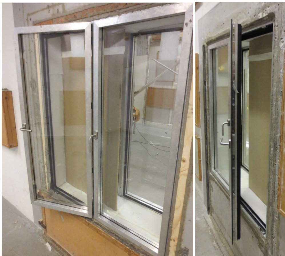
Illustration 8J. Photos of the simulated one-winged sidehung solution without absorbers on the transversal plate.
