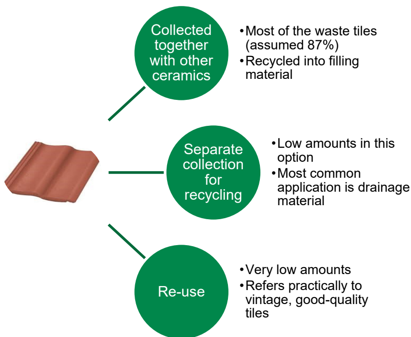
Figure 2.1 Current waste treatment options for roof tile waste in Denmark
