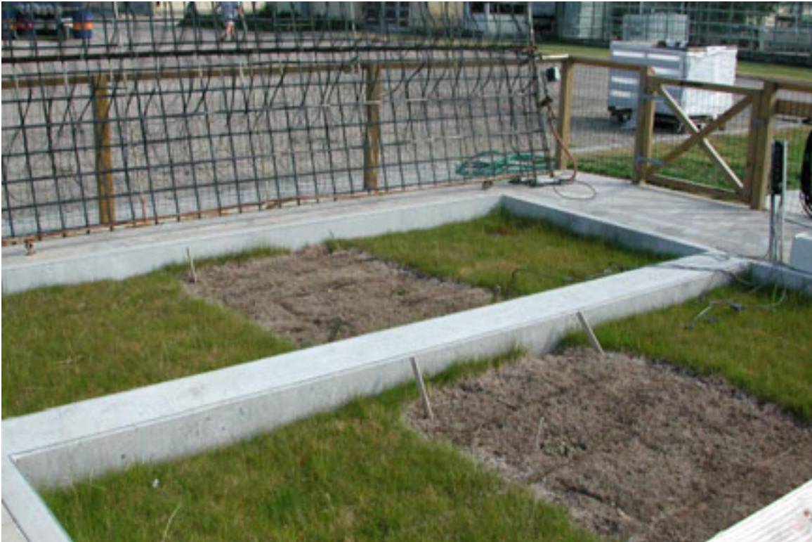
Figure 6. Clear pesticidedamage on the grass shown in august. The frame in the background is used to apply lack of water. To the right is shown electric cables collected to TDR probes to determine water content and instruments for temperature recording
