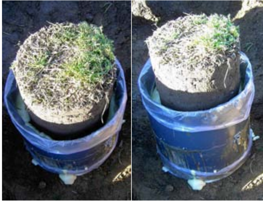
Figur 1.3. Indstøbning af intakt jordkolonne i polyurethancelplast. Figure 1.3. Fixation of naturally layered soil column in polyurethane.
