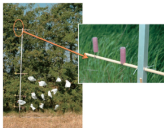
Fig. 2. Photo of mast mounted with curlers and branches covered with plastic bags to avoid untimely exposure. Insert shows closer view of hair curlers on mast.
