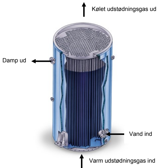
Figur 5: Røgrørskedel af typen XS (Exhaust Smoke tube).
