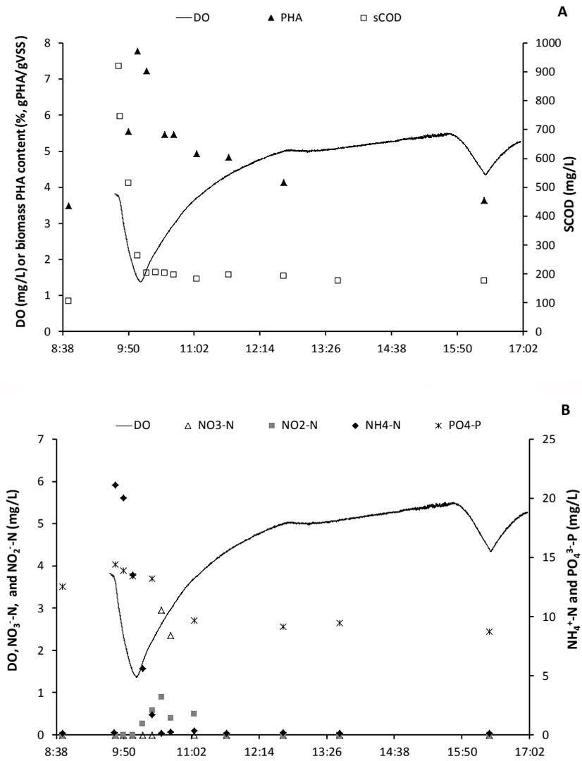
Fig. 10. Characteristic feast-famine cycles with nutrient addition at the start of the feast (2015.06.24). DO profiles with respect to COD and biomass PHA content profiles (A), and DO profiles with respect to N and P profiles (B).
