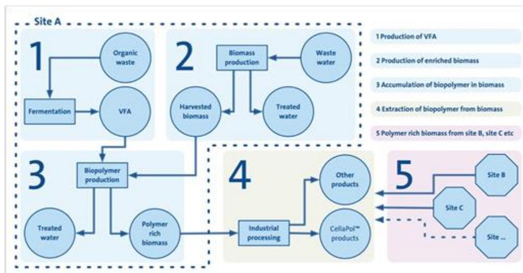
Fig. 2. Process elements (PEs) for the integration of Cella™ Technologies to waste and residuals management
