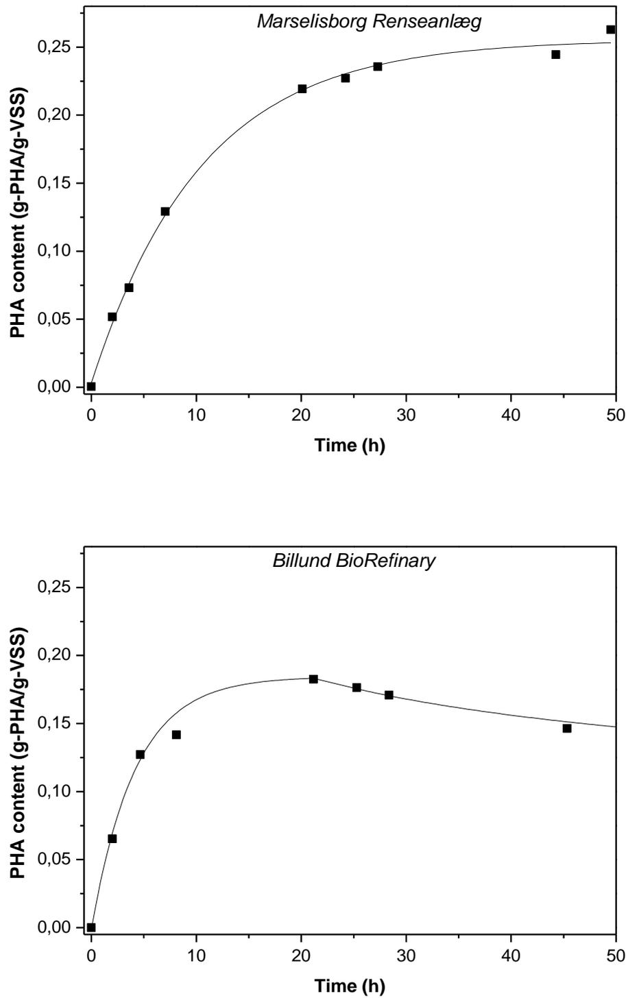
Figure 8. Biomass PHA content during the accumulation test with activated sludge from Marselisborg Renseanlæg and Billund BioRefinery.
