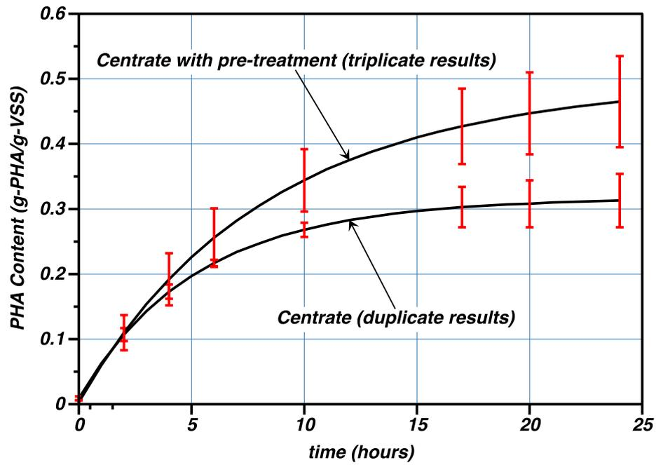
Figure 5. Summarized pilot scale PHA accumulation results with RWZI Bath biomass for replicate PAP assessments using fermented sludge centrate for VFA feedstock, with and without pre-treatment for reducing feedstock phosphorus content.
