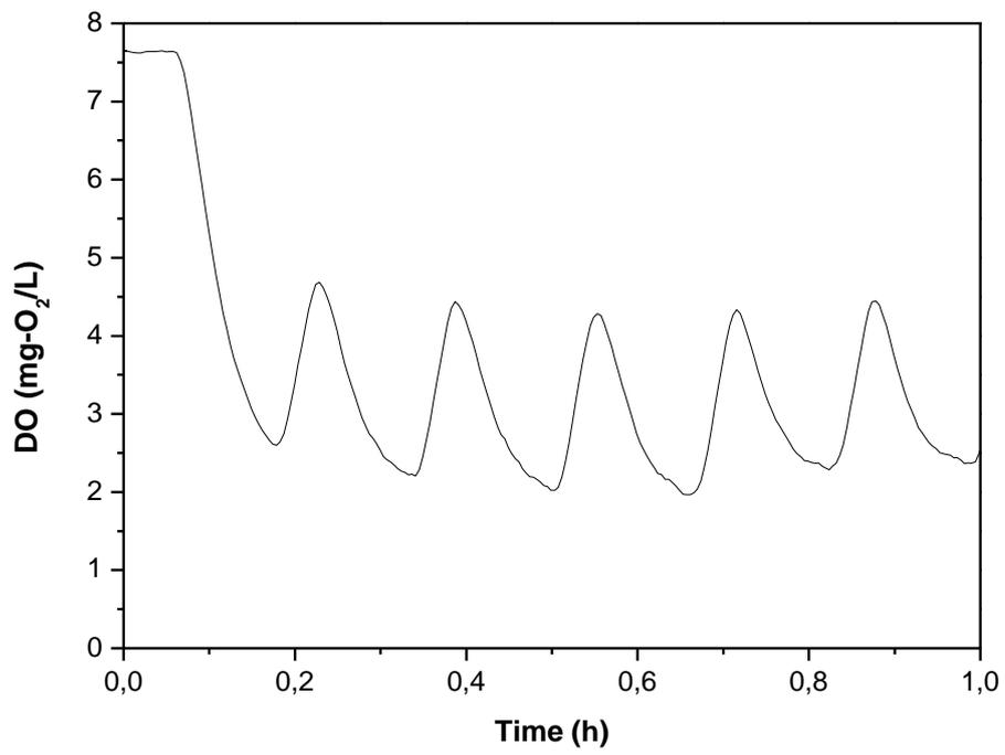
Figure 7. Typical DO concentration curve during the accumulation phases.
