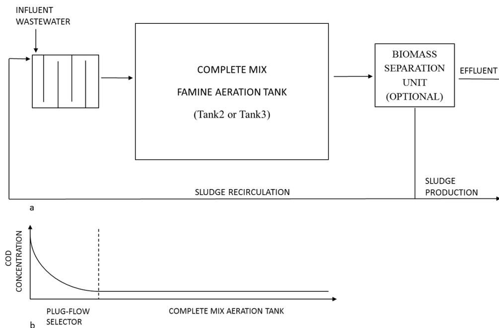
Figures 5. Configuration (a) and COD profiles (b) of KMC process effluent treatment with continuous flows characterized by a selector feast reactor (high F/M) and a famine reactor volume (low F/M).
