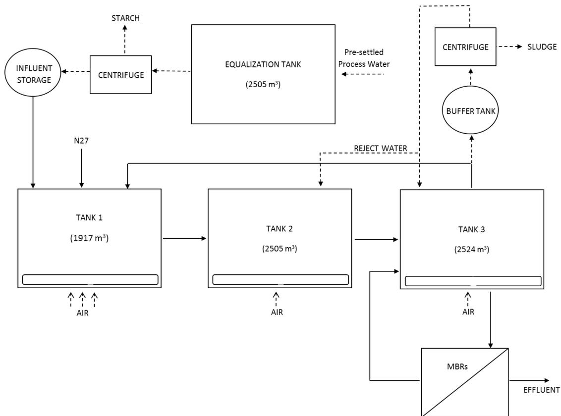
Figure 1. Current configuration (December 2015) of the KMC process water effluent treatment plant. Dashed lines represent semi-continuous flows
