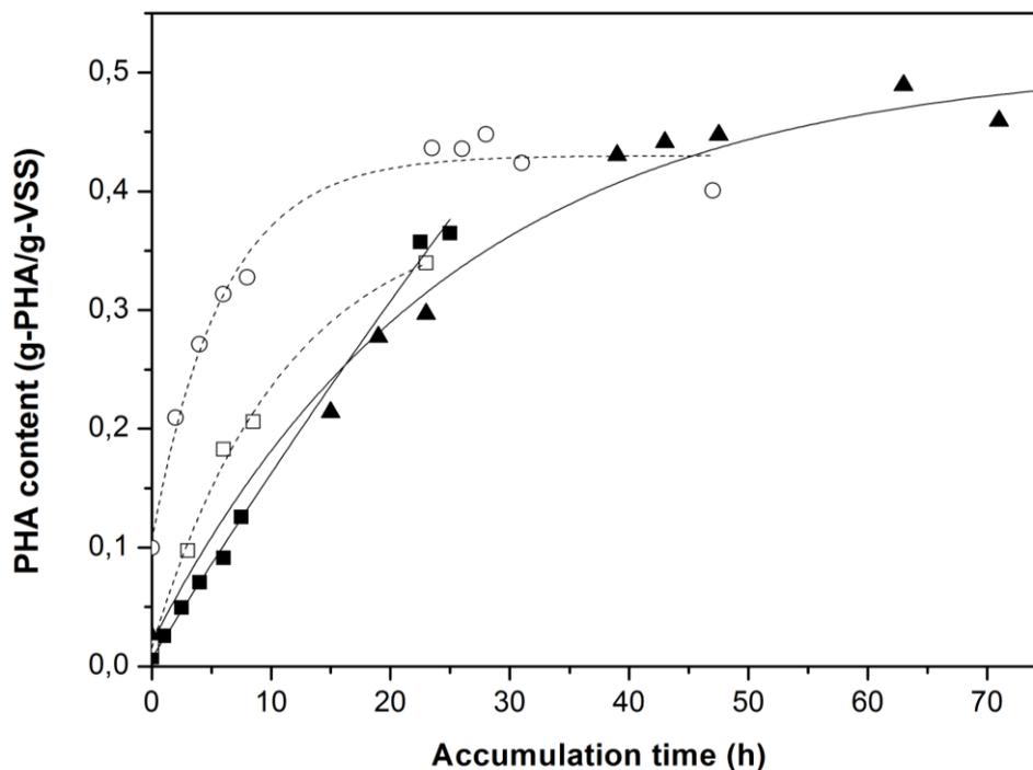
Figure 2. Replicate PAP evaluations for Leeuwarden Cella™ biomass using a reference substrate based on acetate (■ and ▲) and fermented agro-industry centrate (□ and ○) as feedstocks.
