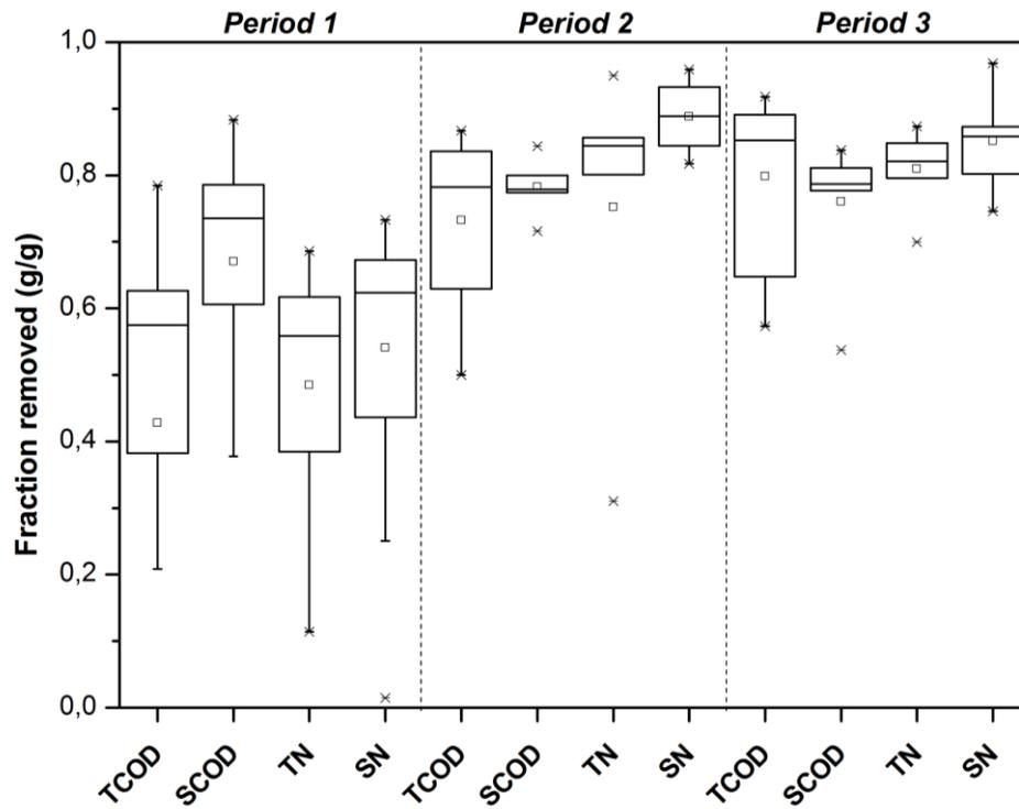
**Figure 3. Removal efficiencies of COD and total N in three operational periods where Period 1 represents a process of pre-denitrification-nitrification and Period 3 represents the same process with an additional element of post-denitrification.**
