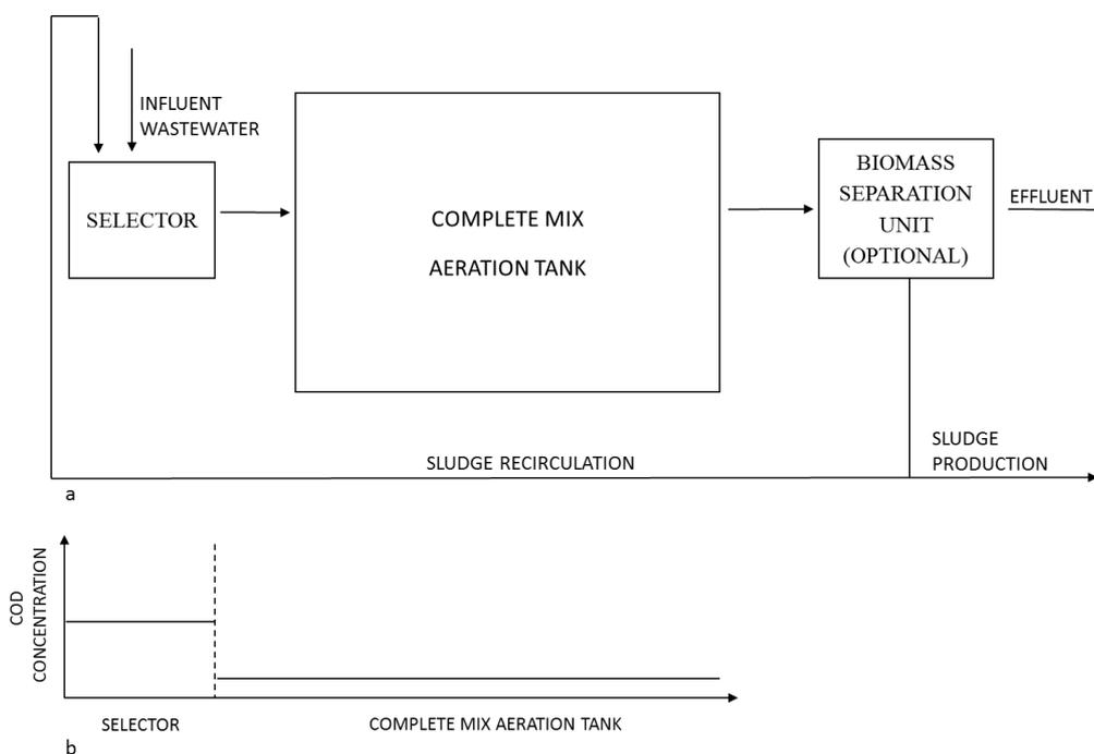
Figures 3. Configuration (a) and COD profiles (b) of a biological treatment plant with selector strategy for sludge bulking control. In this configuration the selector operates under complete-mix conditions.
