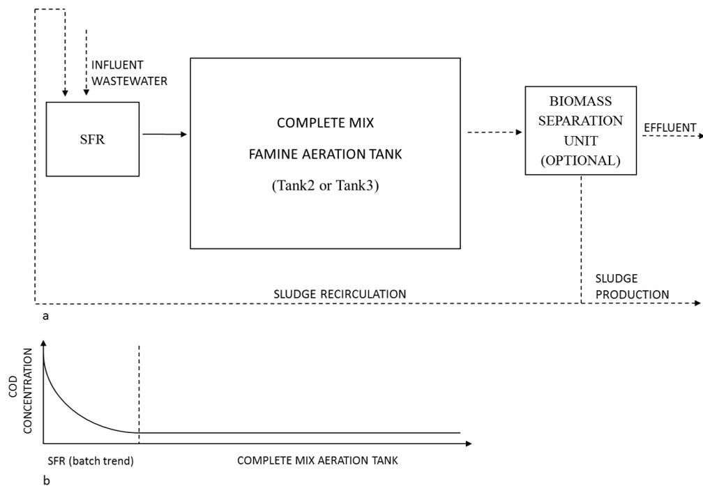
Figures 4. Configuration (a) and COD profiles (b) of KMC process effluent treatment with semi-continuous flows characterized by a sequencing feast reactor (high F/M) and a famine reactor volume (low F/M). Dash lines (a) represent semi-continuous flows.
