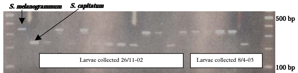
Figure 3.4. Agarose-gel with PCR-products from adult S. melanogrammum (first arrow) and S. capitatum (second arrow) plus unidentified Strophosoma spp. larvae. DNA from S. melanogrammum and S. capitatum gave a band at approx. 350 bp and 250 bp, respectively, using the primer combination Start Stroph. + End-sc4+End-sm3
