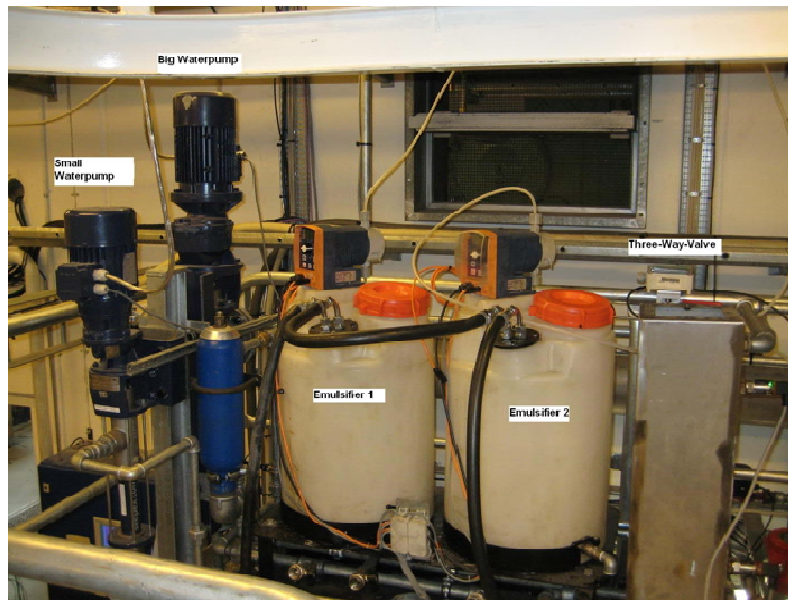
Figure 32 Emulsifier tanks with emulsifier dosage pumps on top. Shown are also the water pumps as well as the three-way valve controlling the addition of emulsifier to either fuel or water.
