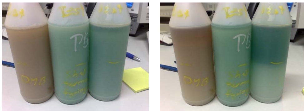
Figure 12 Tests of emulsion stability of MGO and MDO. The bottle with the brownish content is the DMB fuel with a temperature of 22°C with a viscosity of 5 cSt at 40°C, the bottle in the middle is the MGO at a temperature of 5°C, and the bottle to the left is MGO at a temperature of 22°C. The water content in all bottles is approx. 50 vol. % on a total basis. The left image is at t=0 and the right image is at t=2 min.
