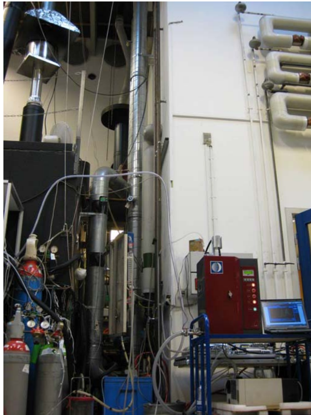
Figure 2. Sampling of particles in wood smoke with ELPI at TI's test plant in Aarhus.
