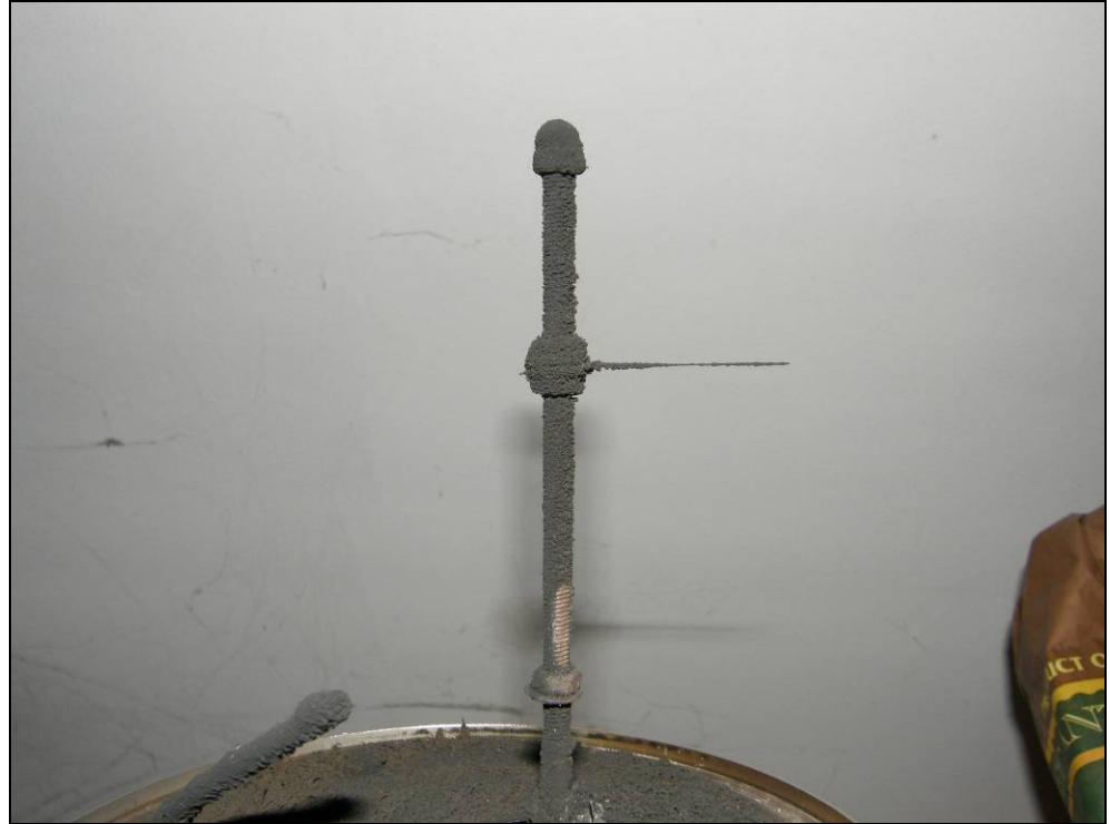
Figure 58. The Zumikon electrode with only app. 5 cm remaining of the original 25 cm
