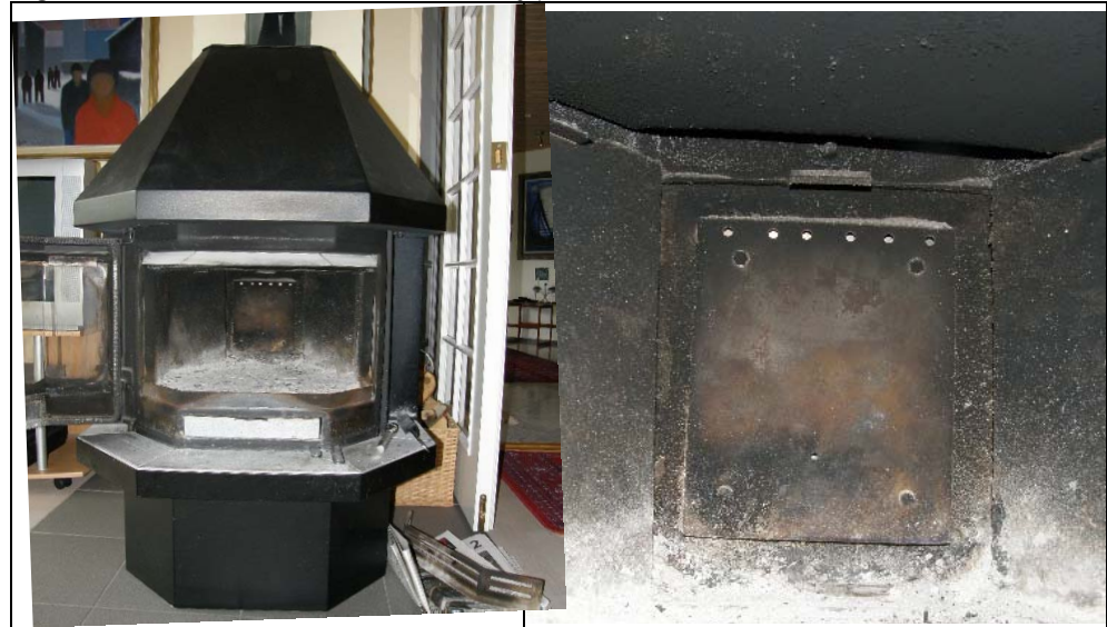
Figure 60. Handöl 10 stove and the Ecoxy plate mounted inside on the back wall
