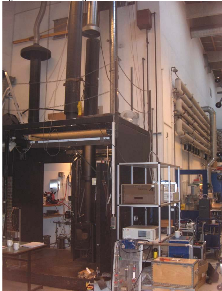
Figure 10. Entire test rig with dilution tunnel
