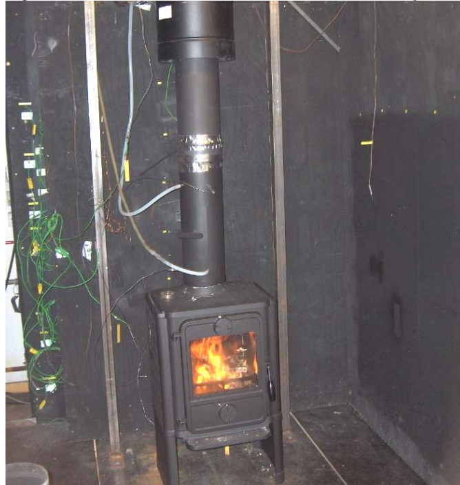
Figure 15. Morsø wood stove with the Morecat catalyst
