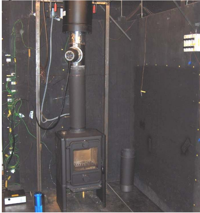
Figure 16. Morsø wood stove with the Zumikon ESP
