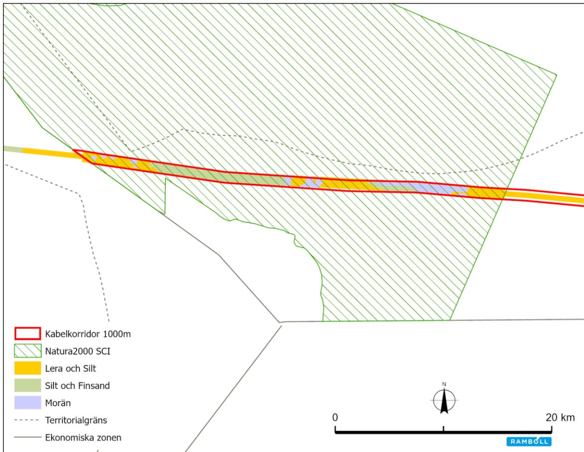
**Figure 11-4. Sediment on the seabed based on sampling in the cable corridor.**
