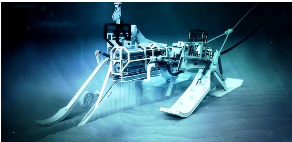
**Figure 3-4. Example of a marine plough (Primo Marine, 2022).**
