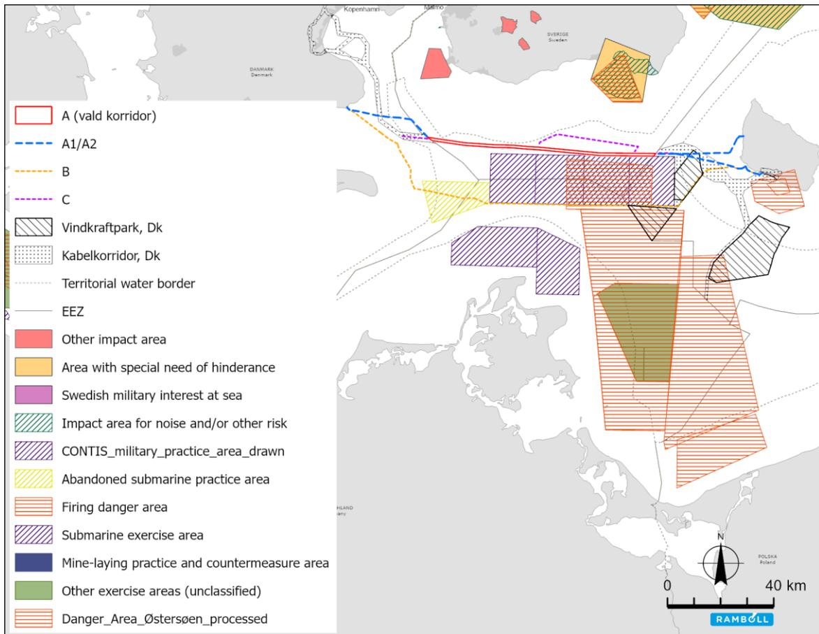
**Figure 5-2. Studied alternative locations for the cable route between Energy Island Bornholm and Zeeland, including areas of military interests. CONTIS military area corresponds to the NATO area described in the text. The selected cable corridor within Swedish EEZ and planning areas for subsea cables, offshore windfarms and onshore areas are also shown.**
