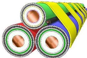
**Figure 3-2. The bundle configuration of the cable systems will consist of four cables: two HVDC cables, a metal return and a fibre optic cable.**
