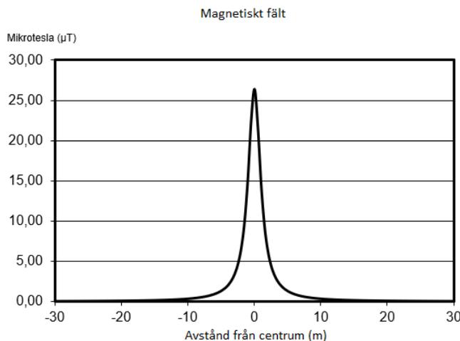
Figure 8-1. The graph shows how the magnetic field rapidly decreases as the distance increases.
