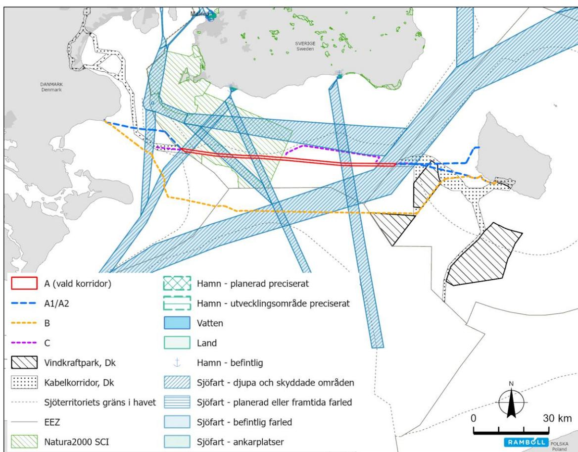
**Figure 5-1. Studied alternative locations for the cable route between Energy Island Bornholm and Zealand, including ship traffic interests and Natura 2000 sites. The selected cable corridor within Swedish EEZ and planning areas for subsea cables, offshore windfarms and onshore areas are also shown.**
