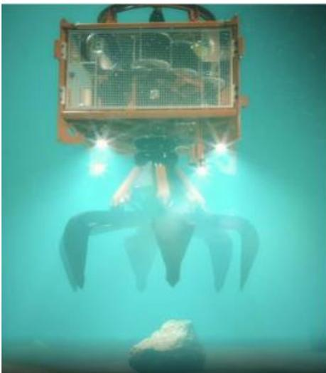
Figure 3-3. Equipment for removing obstacles such as boulders.
