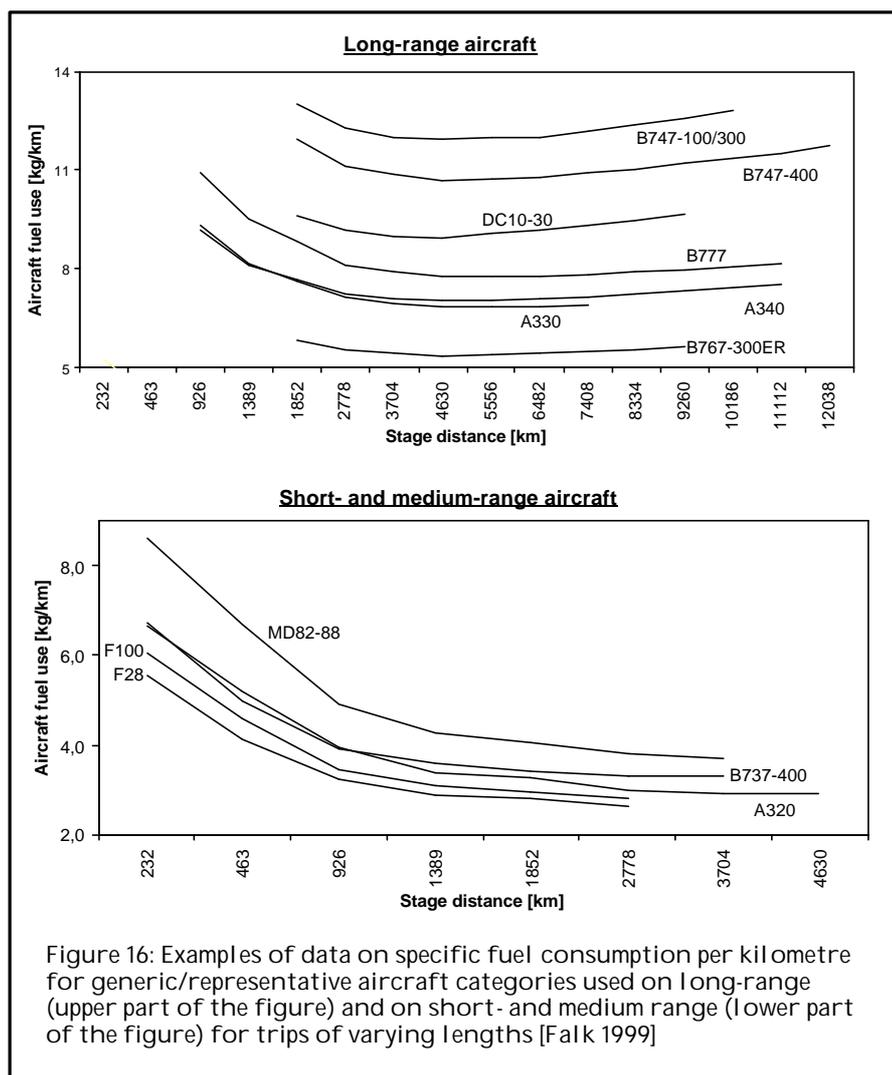
Figure 16: Examples of data on specific fuel consumption per kilometre for generic/representative aircraft categories used on long-range (upper part of the figure) and on short- and medium range (lower part of the figure) for trips of varying lengths [Falk 1999]
