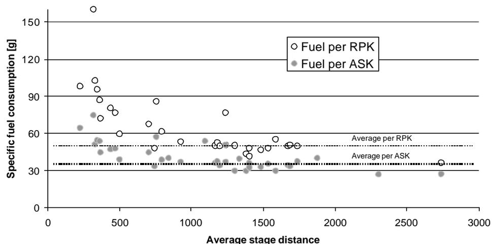
Figure 21: Illustration of the specific fuel consumption per ASK and RPK of American air carriers in domestic operations in 1999
