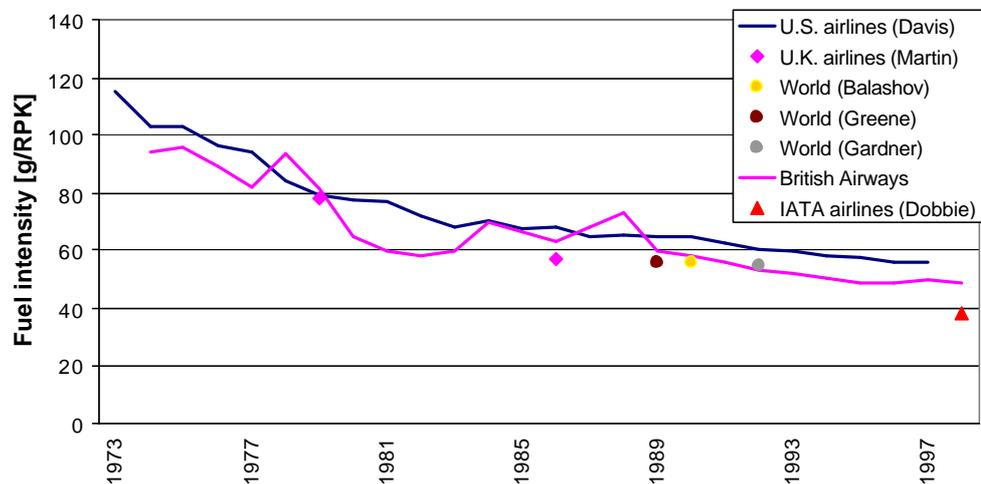
Figure 18: Fuel intensity per revenue passenger kilometre (RPK) of passenger air travel according to various sources [Davis 1999], [Martin and shock 1989], [Balashov and Smith 1992], [Greene 1990], [Gardner et. al. 1998], [British Airways 1999a] and [Dobbie 2001].
