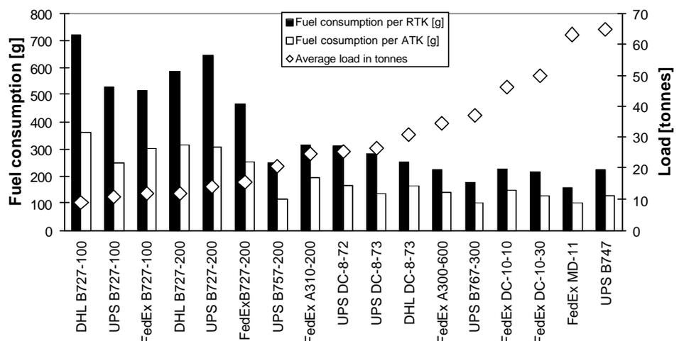
Figure 20: The specific fuel consumption of the main aircraft models operated by the three major US all-cargo carriers in 1998
