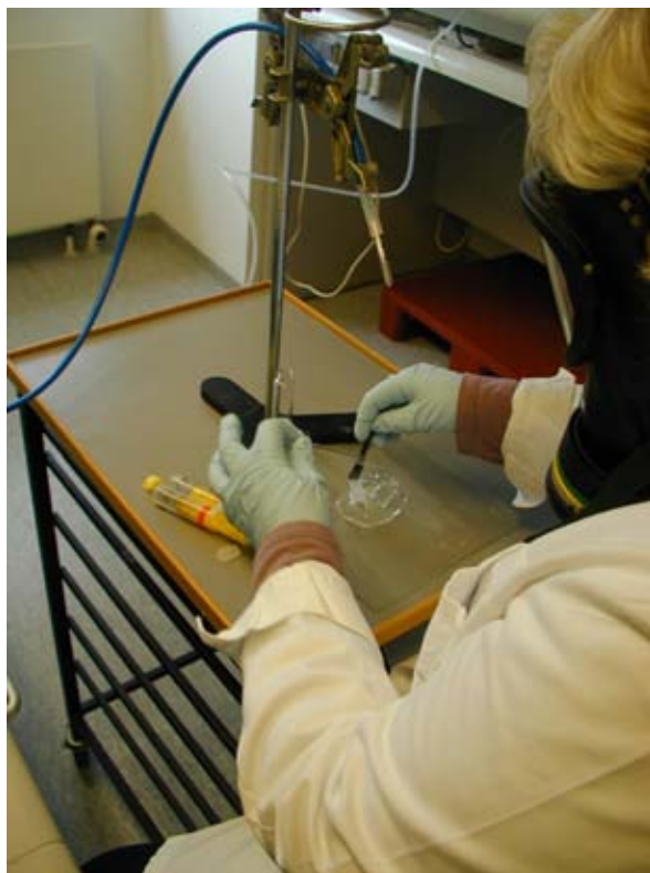
Figure 5: Application of epoxy adhesive. Air is sucked through an XAD-2 column, which is placed in nose height above the work surface.
