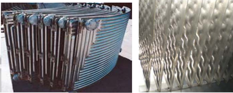
FIGURE 6-4 STRUCTURE OF SELF-CLEANING PLATE HEAT EXCHANGER
