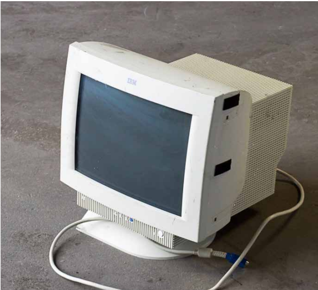
An example of a CRT-monitor. Export of used CRT's is not recommended due to the content of hazardous substances and obsolete technology.
