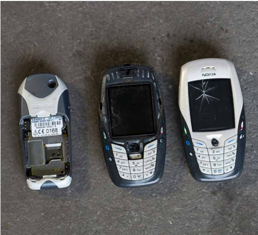
Examples of mobilephones with serious signs of wear and missing components that hinder functionality.
