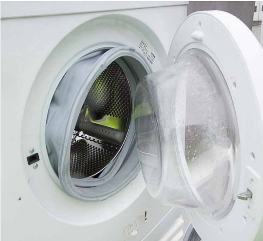
An example of a washing machine which show serious signs of wear. The seal on the door is damaged in such a way that it hinders functionality.
