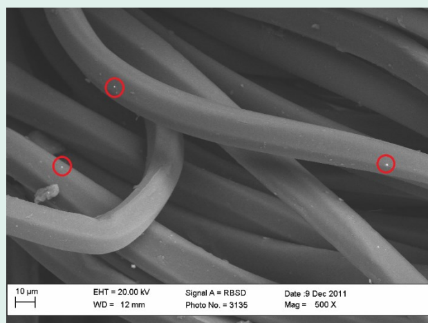
Scanning electron microscopy (SEM) of nanosilver particles marked by red circles on fibres from the inner sole of a sandal [3]
