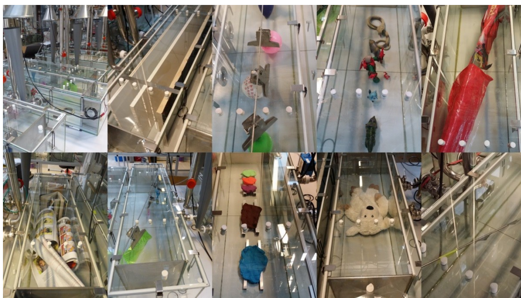
FIGURE 6.3. SETUP IN CLIMPAQ CHAMBERS. FROM THE LEFT, TOP: CLIMPAQ CHAMBERS AT SBI, WALL AND WOOD PAINT USED ON GIPSUMBOARD AND WOODEN BOARD, BALLOONS, RUBBER FIGURES, PLAY TENT, DOWN: COMICS, RUBBER BEACH-ARTICLES, MODELLING CLAY, TEDDY BEAR, TAPE
