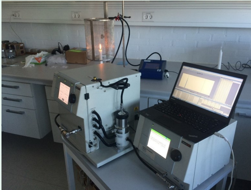
Figure 4 Measurement set-up during measurement of particle emissions from candles with SMPS.
