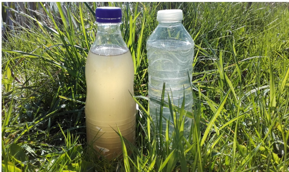
Figure 6.3 – Water from the filtration process. The bottle on the left (blue cap) contains a sample of ingoing water, while the bottle on the right (clear cap) contains filtered water.
