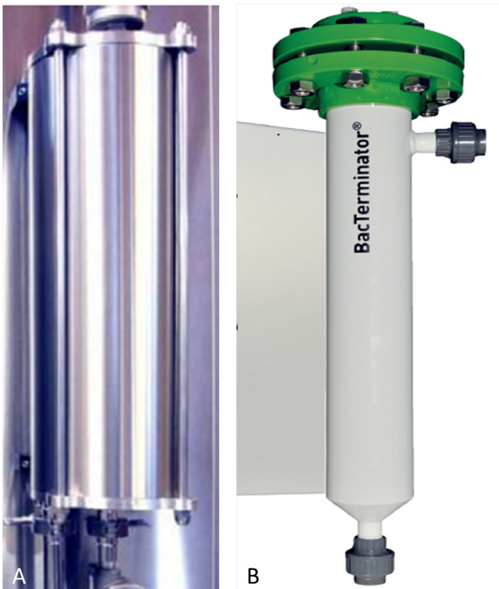
Figure 7.3 - Pictures of the old AO system (A) and the new design (B). In the old system metal parts cover 4 plastic parts, which are kept together by nuts and bolts. The new and larger design version uses bolts to keep the top to the chamber.
