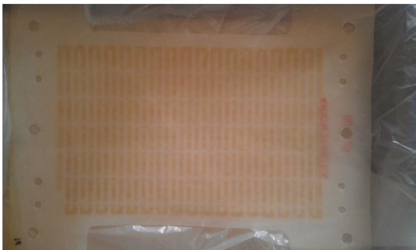
FIGURE 21. THE ANION EXCHANGE MEMBRANES AFTER CLEANING AND EXPERIMENTS IN THE BENCHSCALE STACK.
