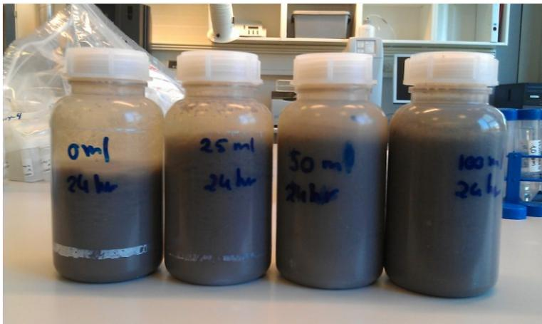
FIGURE 9. THE 4 BOTTLES OF SECONDARY SEWAGE SLUDGE AFTER 24 HOURS CONTAINING 0, 25, 50 AND 100 ML OF 48 HOUR HYDROLYZED PRIMARY SLUDGE.
