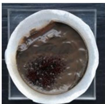
FIGURE 4. FOULING AND SUBSEQUENT BURNING OF AN ANION-EXCHANGE MEMBRANE BY TRANSPORT OF ORGANIC MATTER ONTO THE SURFACE AND INTO THE PORES.
