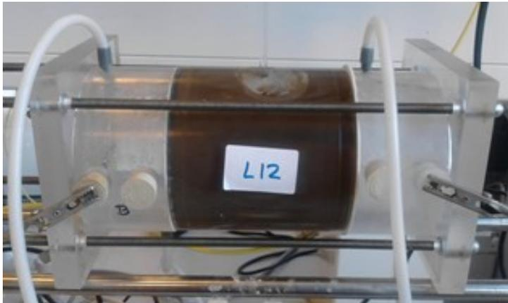
FIGURE 14. THE LABORATORY SCALE 3-COMPARTMENT ELECTRODIALYTIC CELL SETUP AS USED IN THE LABSCALE EXPERIMENTS.
