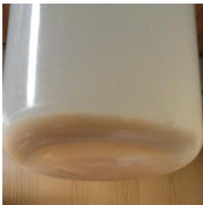
FIGURE 22. THE (VISIBLE) ORGANIC MATTER RESIDUE THAT WAS RETRIEVED FROM THE MEMBRANES AFTER RINSING WITH A 1 LITER 5% NAOH SOLUTION.
