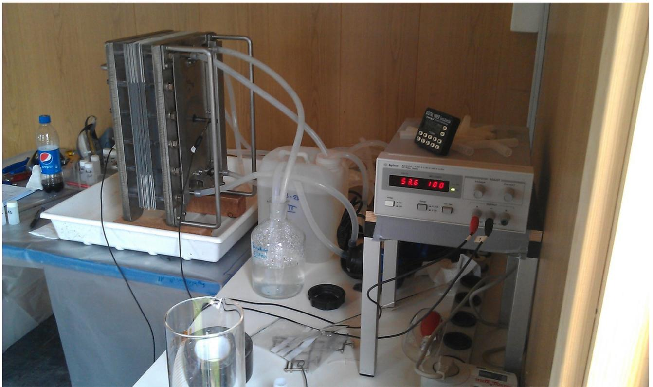
FIGURE 17. A PHOTO OF THE BENCHSCALE ELECTRODIALYTIC CELL SETUP AS USED IN THE EXPERIMENTS. THE ELECTRODIALYSIS STACK IS TO THE LEFT.
