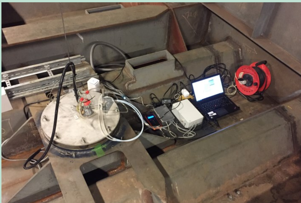
FIGURE 27. Measurement setup at the central node lamp outlet during the CO 2 campaign
