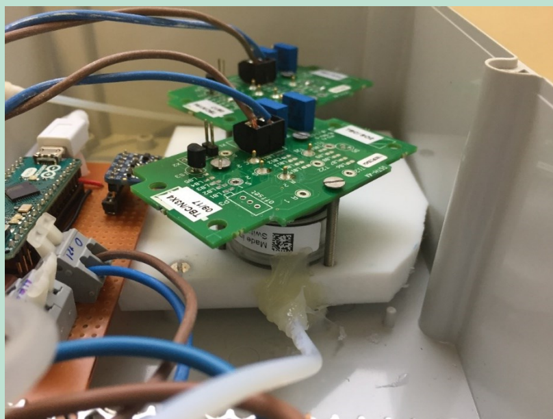
FIGURE 21. The build of the flow through setup for the electrochemical sensors. The white block is PTFE (Teflon) in order to be chemically resistant to the plume gas.
