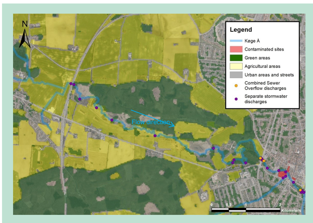
FIGURE 12. Identification of potential point and diffuse sources of pollution together with the land use pattern close to the stream stretch of interest.
