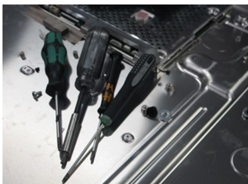
FIGURE 12. picture of some of the different screwdrivers used to separate the television
