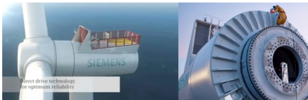
FIGURE 37. Direct drive generator and the magnets
