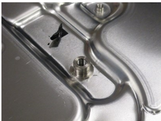
FIGURE 18. Screw thread of iron or stainless steel embedded in aluminium.
