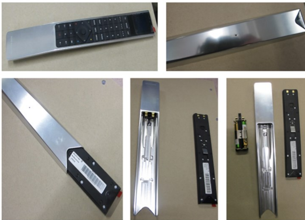
FIGURE 20. Picture of the remote control and the disassembly of the remote control.
