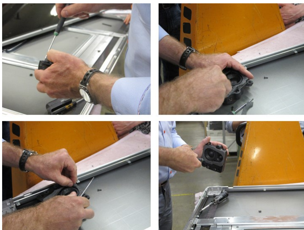
FIGURE 11. Employee from Averhoff working on disassembling a loudspeaker, to examine if it contains neodymium during the workshop
