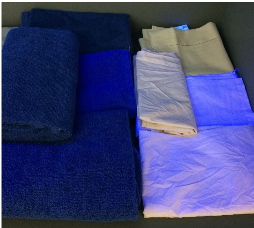
Figure 3-1: Example of visualisation of OBA in non-OBA textile after wash with OBA textiles when exposed to UV light. OBA is detectable by the bluish glow of the textiles.
