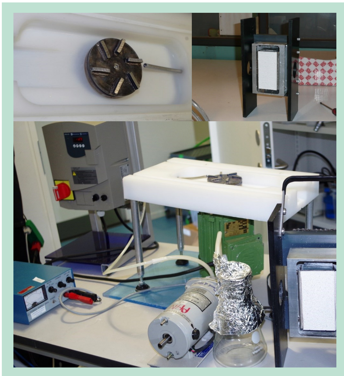
Figure 2.2-2 Grinding machine. Upper left picture: The diamond grinding head. Upper right picture: the sledge holding the render tile. Lower picture: The grinding machine on a lab table.
