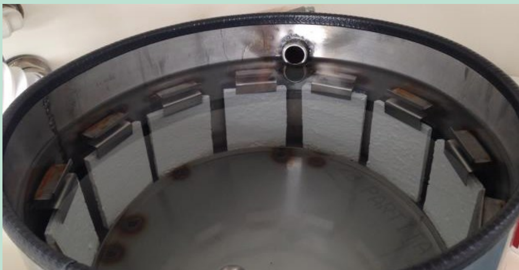
Figure 2.2-3 Setup for creating continuously wet leaching conditions.
