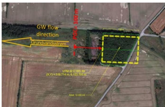
**Figure 32. Conceptual model of the landfill of Hørløkke. The Source term model provides the coordinates; the source length  $L_x$  and width  $L_y$  (yellow dotted rectangles); the groundwater flow direction. The 100 m distance to the point of compliance (POC, red dotted line) is measured from the most downstream point of the landfill.**
