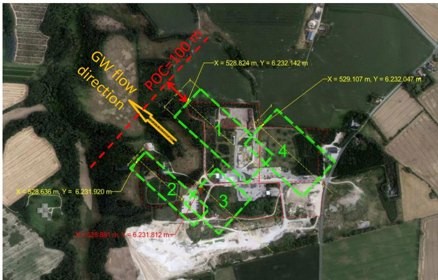
**Figure 18. Conceptual model of Affaldscenter Tandskov. Source length  $L_x$  and width  $L_y$  (green dotted rectangles) and the groundwater flow direction are shown. The 100 m distance to the point of compliance (POC, red dotted line) is measured from the most downstream point of the landfill.**
