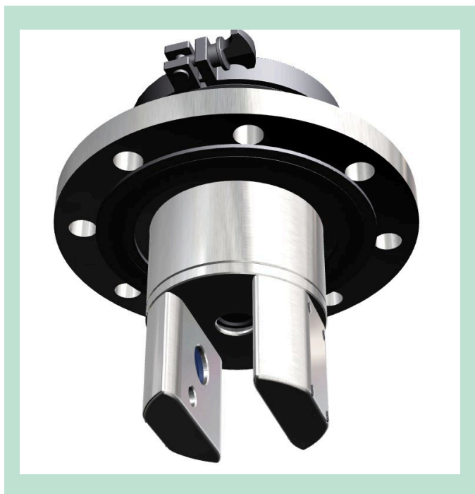
FIGURE 2. bw-monitor unit with two sensors (small and large orifice). The two legs are immersed in ballast water and a standard DIN flange is included for installing in ballast pipe.
