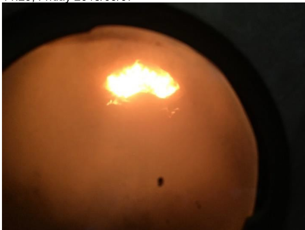
Photo #3: Combustion on difficult rice husks. Ignites at bottom of grate – only combustion on the 2 last grate steps. Ash sample # 1 taken from the end of the grate. At 12:15, Friday 2018/09/07
