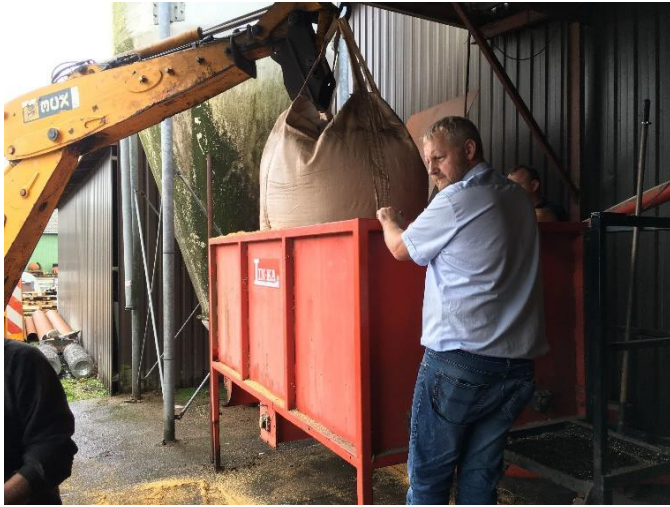
Rice Husks being loaded to fuel bin
