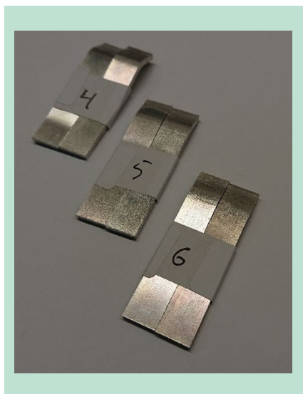
FIGURE 21. Photos of lap shear samples after lap shear testing. Aluminum heat pressed with PMMA. Note that the sample has bended during lap shear testing.
