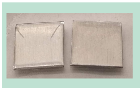
FIGURE 16. Photo of (left) blank and (right) nanoprimed aluminum samples.
